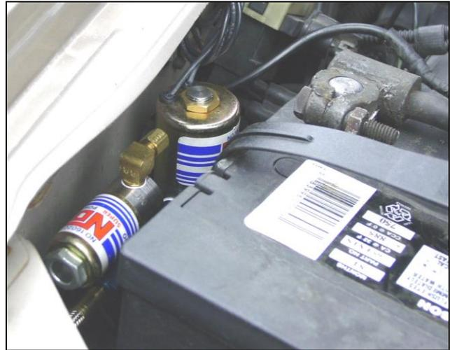
Figure 11 Completed solenoid mounting
