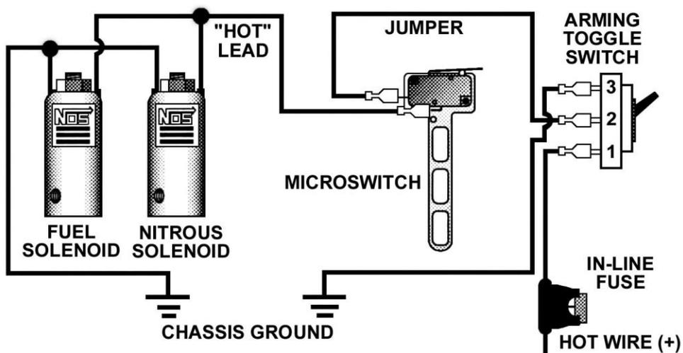
3. Install the arming switch (17) within easy reach of the driver.
