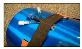
NOTE: The heater element must be in direct contact with the surface of the bottle.
