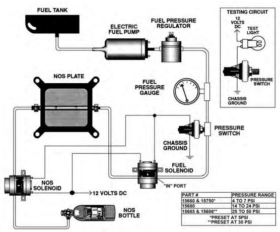
**NOTE:** This schematic is for a nitrous system that draws no more than 10 amps. If this switch is to be used with a system that draws more than 10 amps, a relay must be used.
