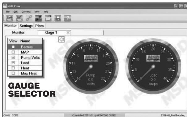
Figure 7 Gauge Selector Box.
