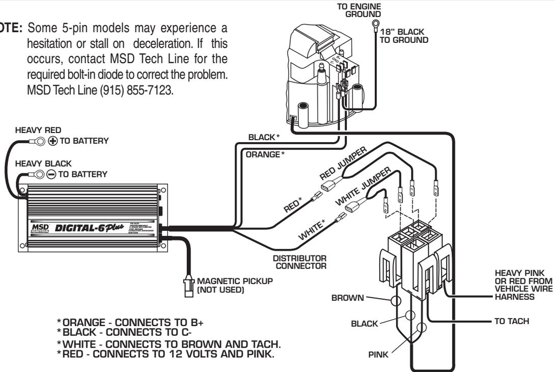
**FORD IGNITIONS Wiring a Ford DuraSpark using White Wire Trigger.**
