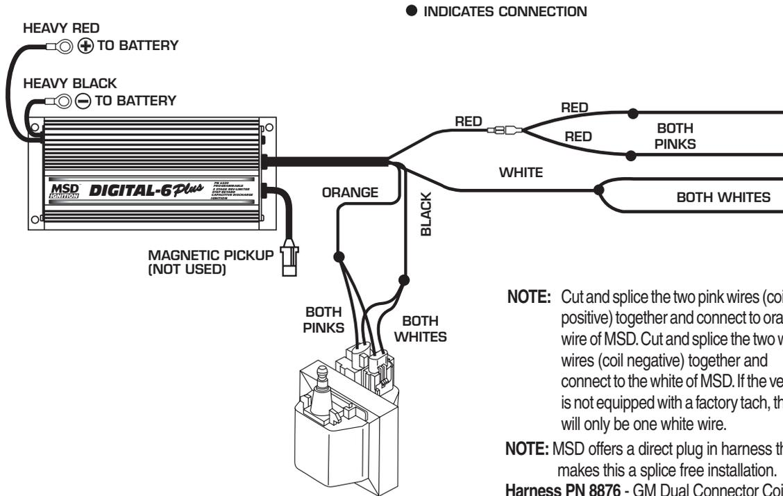
**GM IGNITIONS Wiring the 1996 and up single connector coil without harness.**
