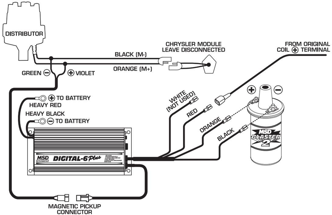
**CHRYSLER IGNITIONS** Wiring a Late Model Dodge with 2-pin connector.
