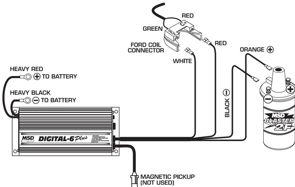
**FORD IGNITIONS Wiring a Ford DuraSpark using Magnetic Pickup Trigger.**
