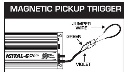
**Figure 12 Checking for Spark with the Mag Pickup.**
