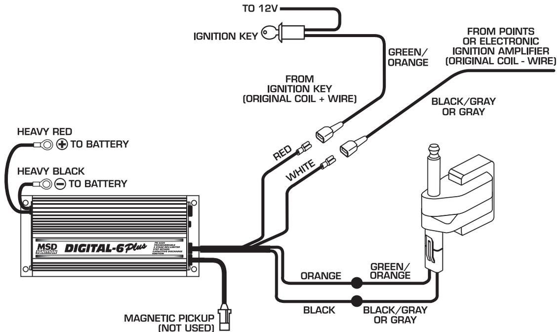
NOTE: Original wiring must be cut.
