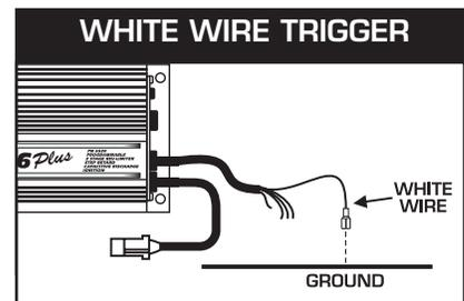
**Figure 11 Checking for Spark with the White Wire.**
