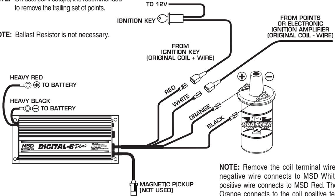
**NOTE:** Remove the coil terminal wires. The negative wire connects to MSD White. The positive wire connects to MSD Red. The MSD Orange connects to the coil positive terminal, Black connects to the coil negative terminal.
