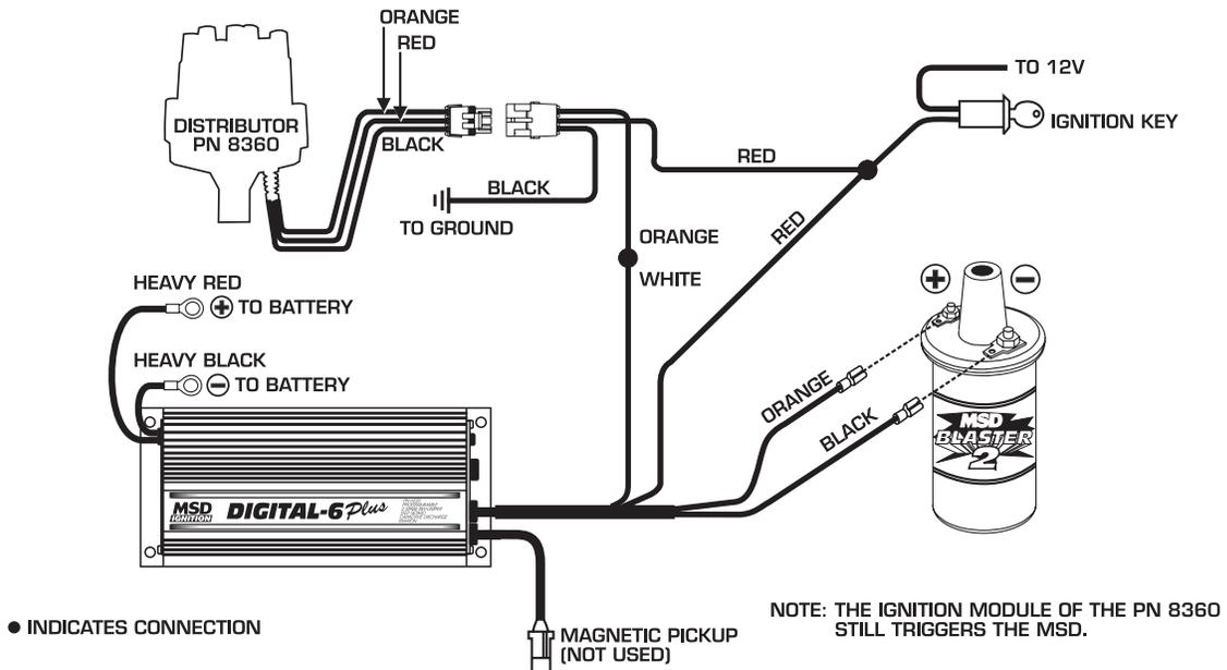
**MSD SYSTEMS Wiring a Complete Dual MSD Ignition Setup.**
