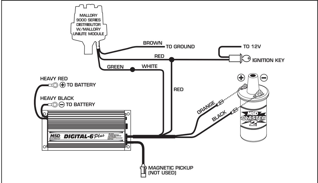
**AFTERMARKET COMPONENTS** Wiring a Mallory 9000 Series using Magnetic Pickup.
