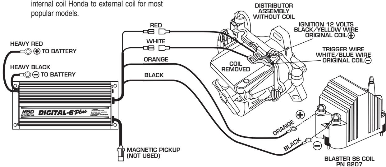
**HONDA IGNITIONS Wiring a Factory External Coil Honda/Acura .**
