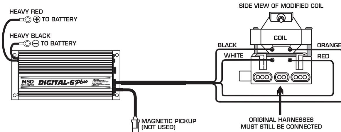
**HONDA IGNITIONS** Wiring a Honda with Internal Coil.
