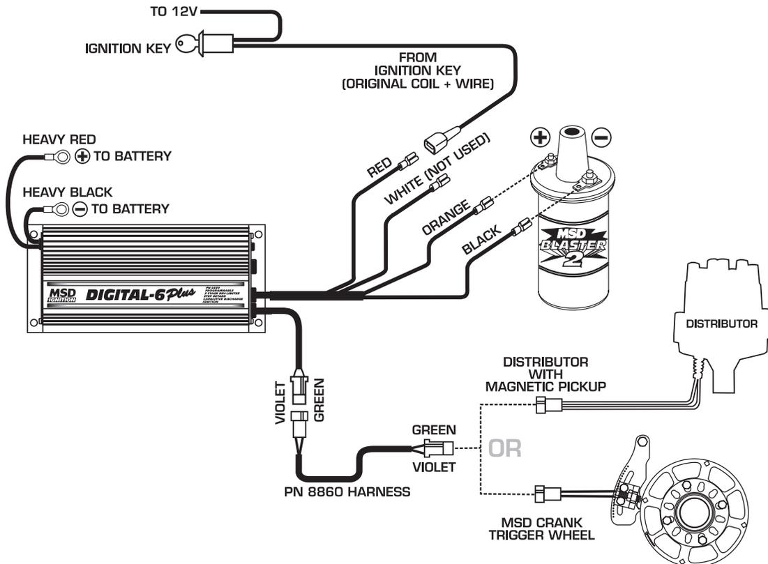
**MSD SYSTEMS Installing to an MSD Distributor PN 8360.**
