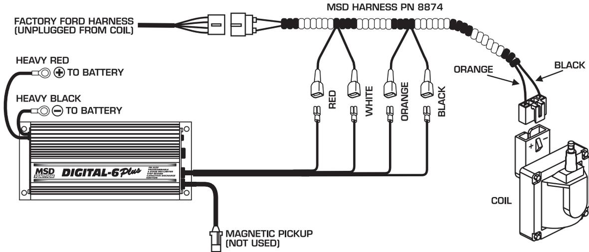
**NOTE:** Installation of a Timing Control with the Harness, see page 15.
