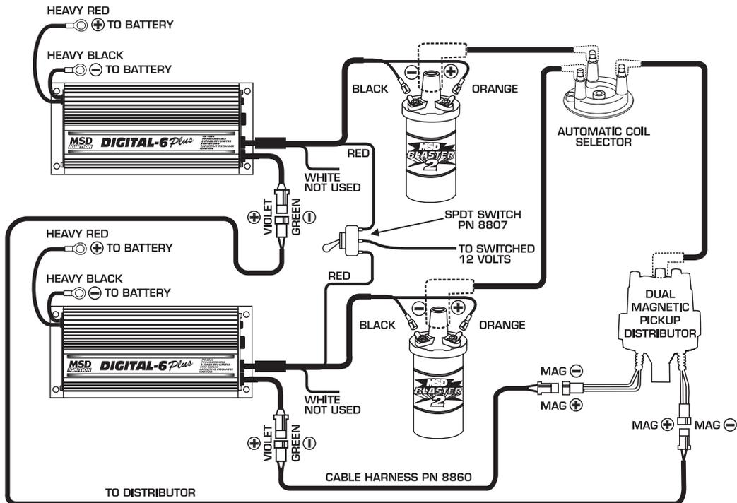
**MSD SYSTEMS With an MSD Timing Control (points or amplifier).**
