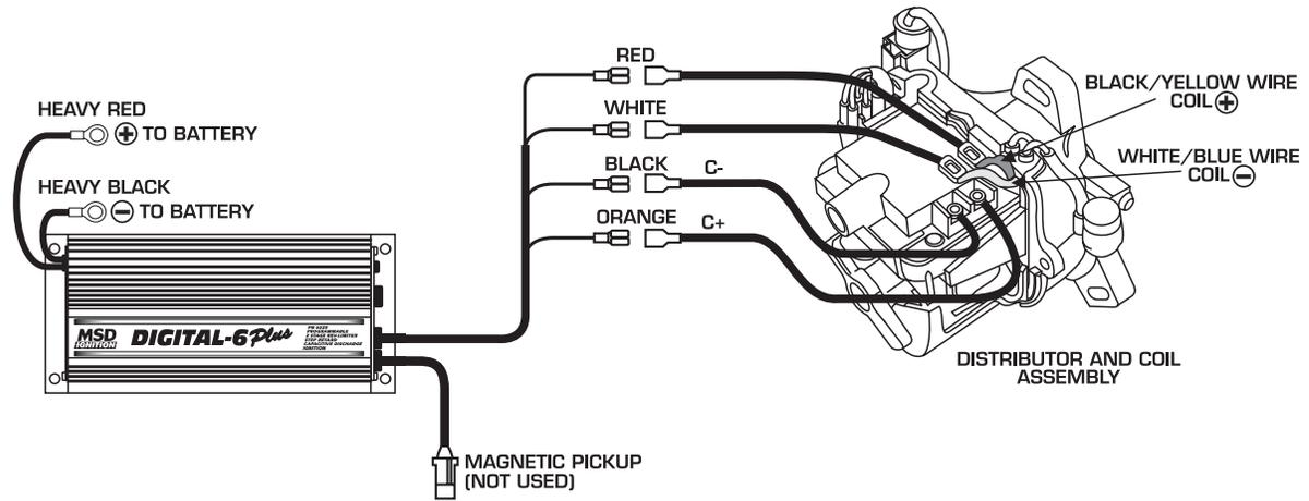
**HONDA IGNITIONS** Wiring a Honda with a Blaster Coil and Power Cap.
