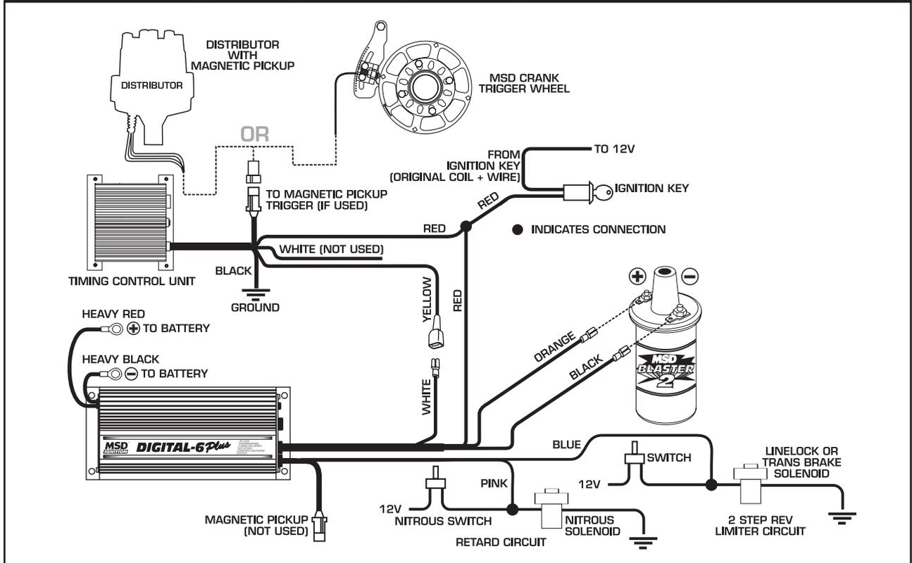
**GM IGNITIONS Wiring a Dual Connector Coil.**
