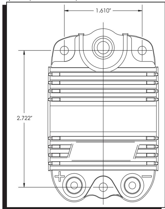
**Figure 1 Mounting Template.**
