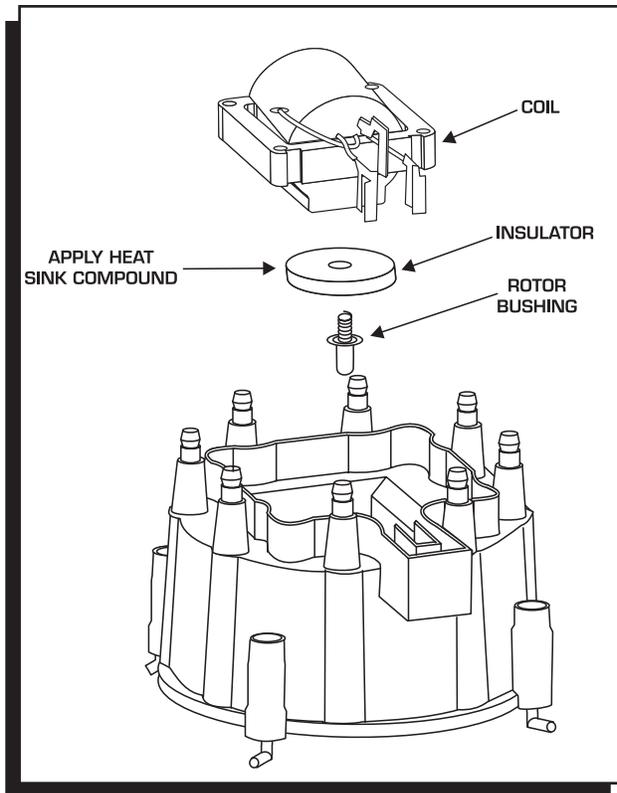
Figure 3 The Coil, Rotor Bushing and Insulator.
