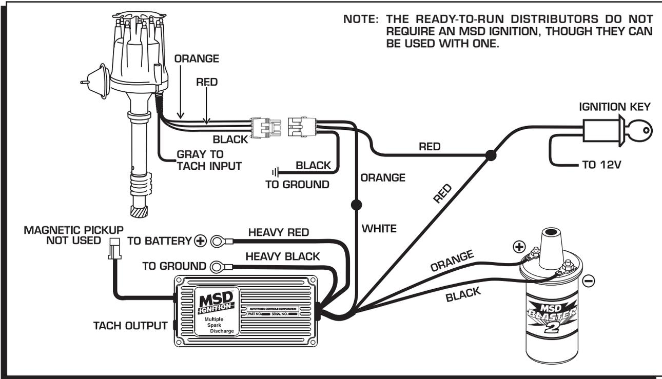
Figure 10 Connecting an MSD Ignition Control to the Ready-to-Run Distributor.
