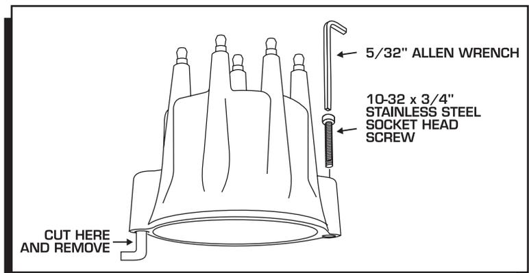
**Figure 14 Optional Installation by Bolting the Cap Down.**
