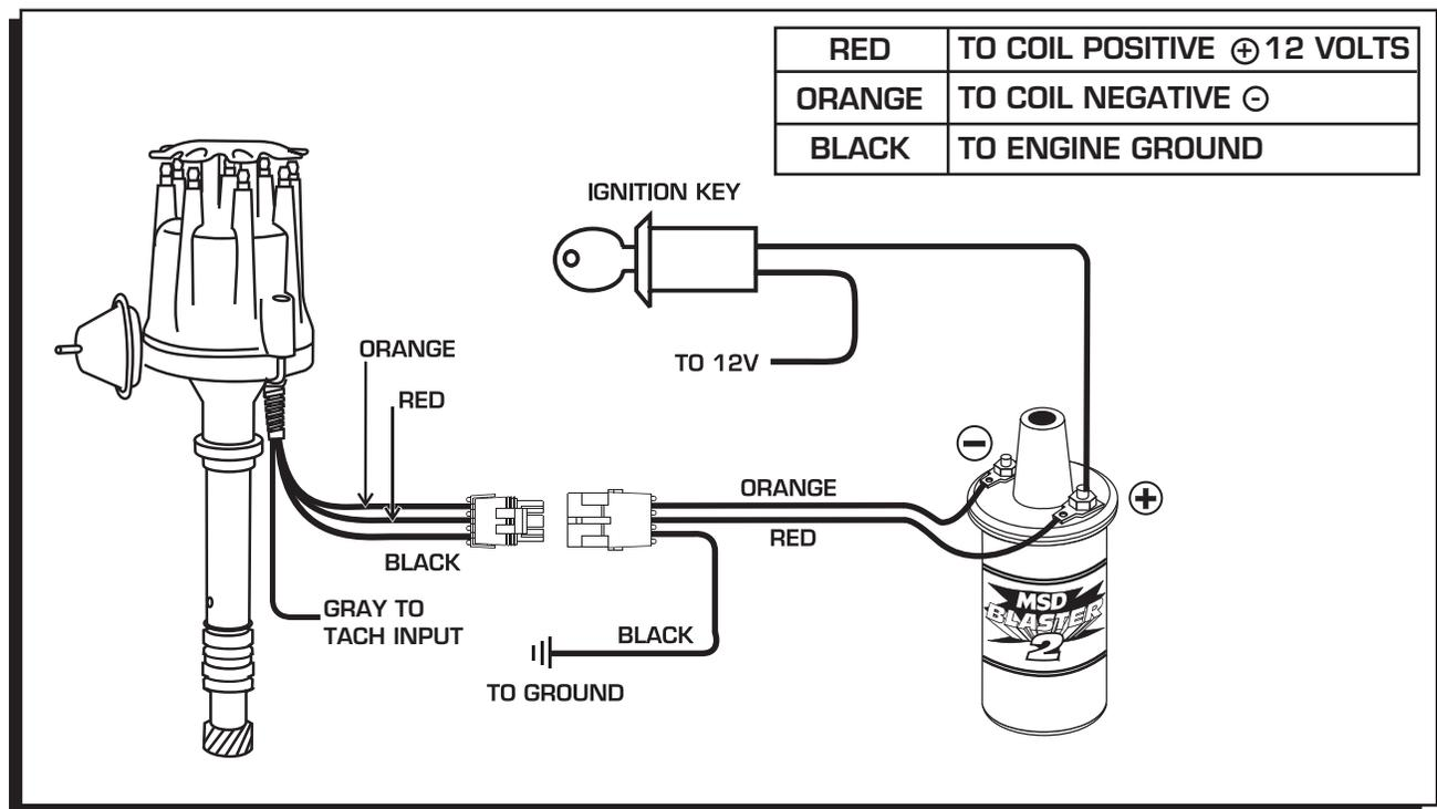
Figure 9 Wiring the Ready-to-Run Chevrolet Distributor.
