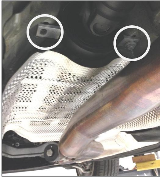
7. Disconnect both swaybar endlinks from the bar and move them out of the way.
