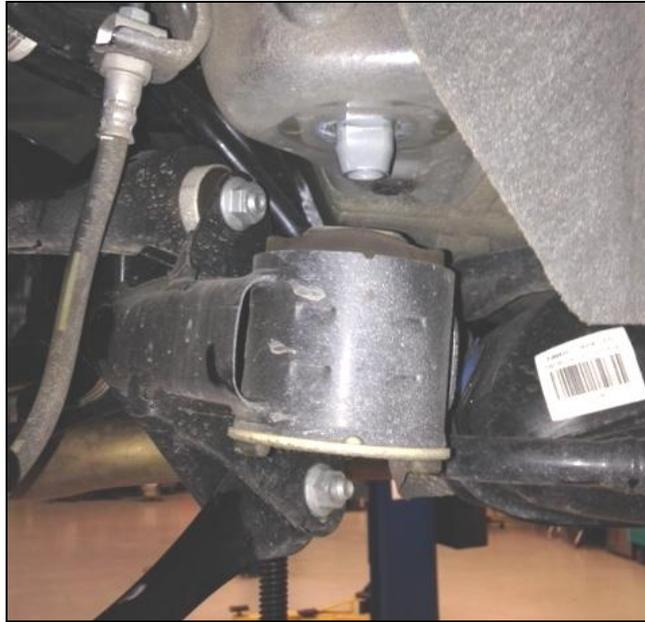
12. Remove the bolts for the swaybar mounts.
