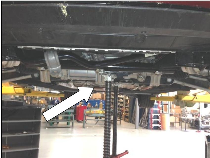
18. Remove the 4 bolts for the front of the subframe.
