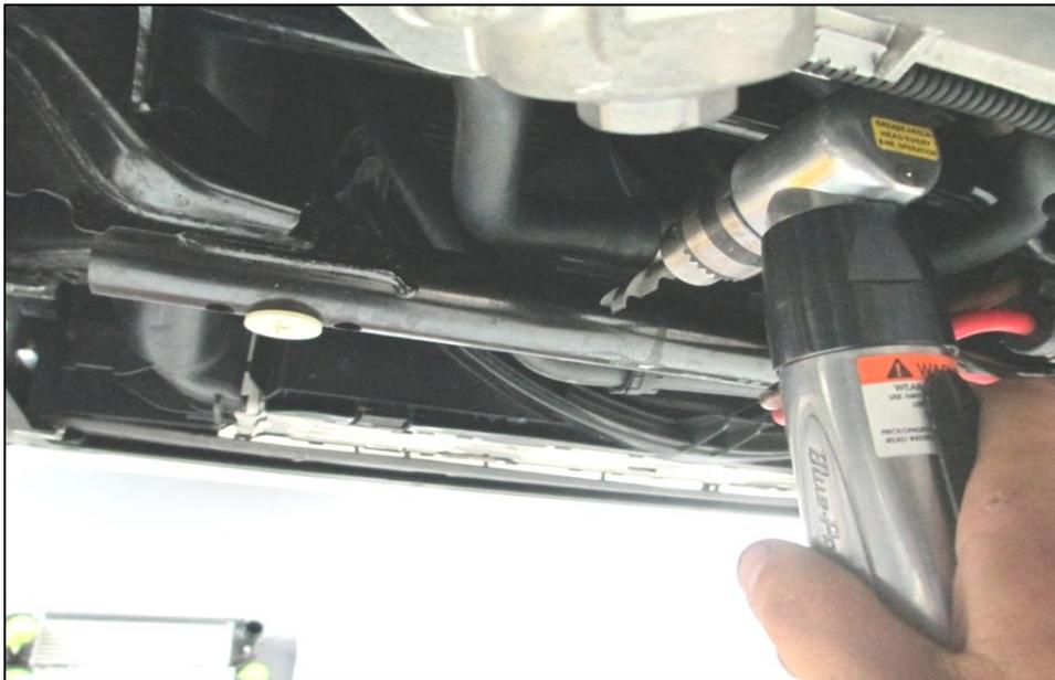
26. Install one of the holders into this hole, and clip the hose into its new location. One holder is adequate to hold this hose.
