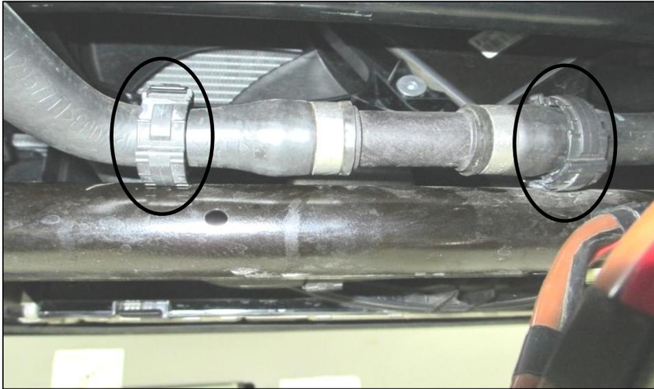
24. Then remove the holders from the subframe by pulling up on the tab to unlock it (see arrow). One of these holders will be reused. The other will be discarded.
