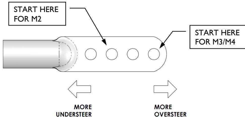
8. The Dinan endlinks must be adjusted to match the length & orientation of the stock endlinks. For easy adjustment, the Dinan end links are left/right hand threaded. Failure to follow the subsequent steps can result in loss of control, vehicle damage, and injury!
