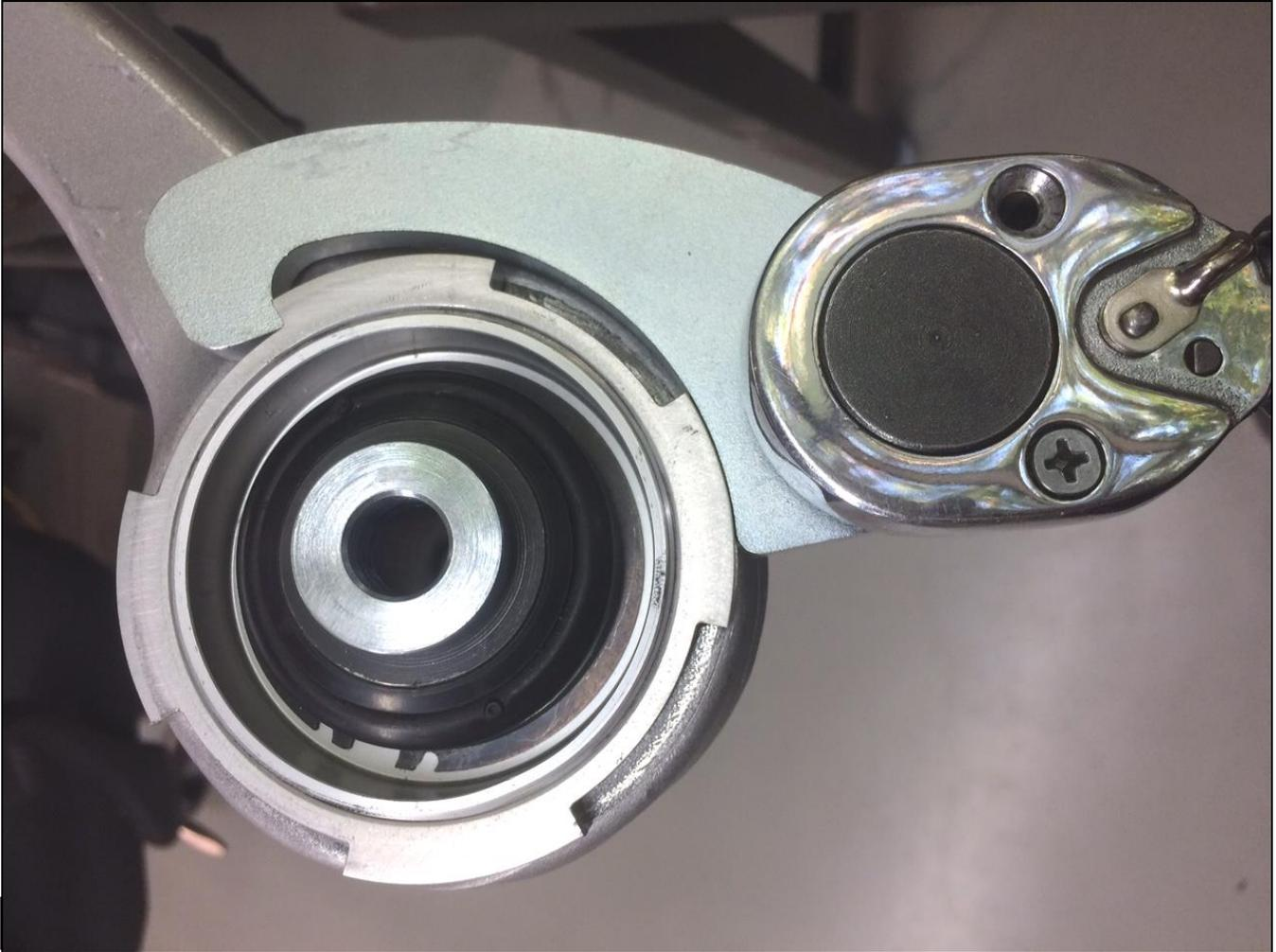
6. Once tightened properly, install the spacers into the ball joint on each side.
