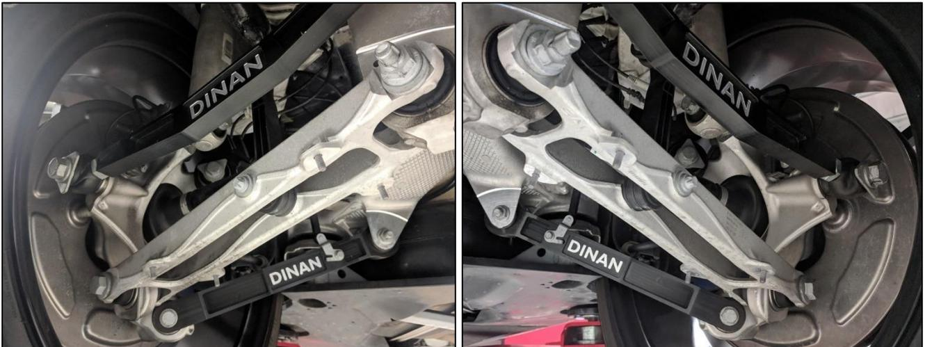
Figure 1: Rear Left Suspension Links (LEFT) and Rear Right Suspensions Links (Right)
