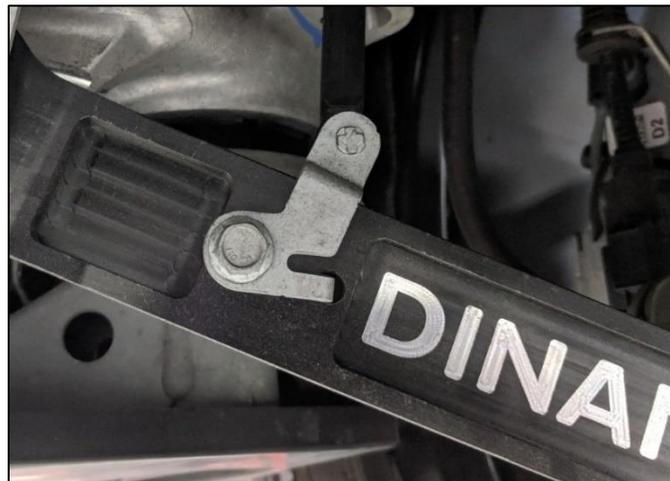
*Figure 4: Ride Height Sensor Installed*
