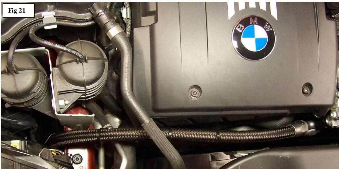
42. Below shows the finished routing of the Hoses. It is critical that you get the mounted angle of the 120° hose end just right so it **does not kink the hose**, and it will line up with the hole you made in the brake duct. Loosely tighten the 120° hose end so it looks like the lower photo for now. Leave sufficient clearance at the circled bracket.
