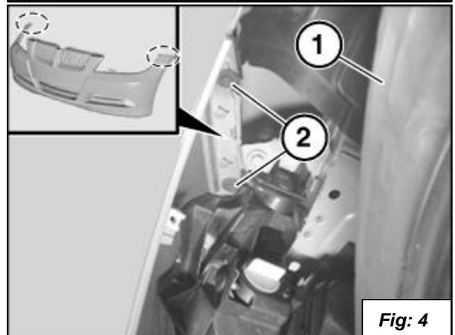
7. Disconnect the fog light connector and parking sensor connector if equipped with them.
