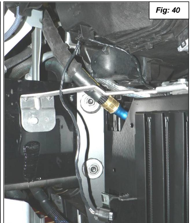
48. Install the bumper over the air duct after connecting the fog light on the passenger side as you install it.
