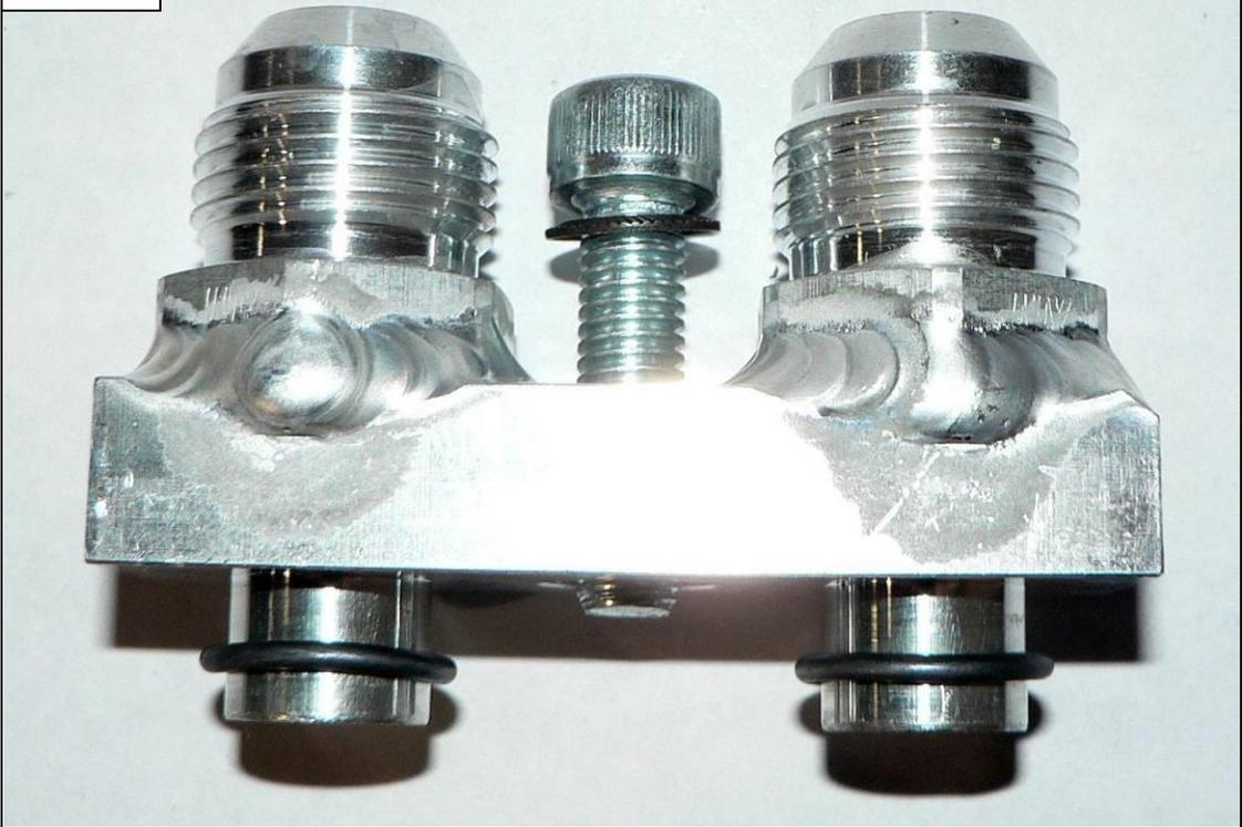
36. Install the oil line adapter block onto the oil filter thermostat housing. Make sure the O-Rings doesn't get pinched as you install the block. Torque the bolt to 20Nm (15ft-lbs.). See figure 30.
