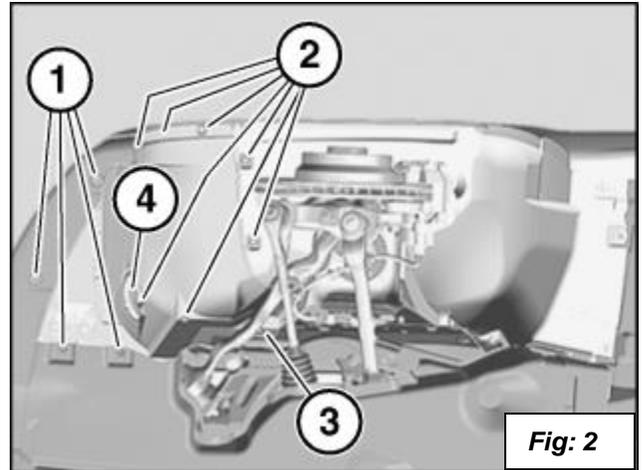
5. On the left side remove the screws in location (1) and pry out the inner fender (2) to gain access to the two screws you will remove in the next step. See figure 3.
