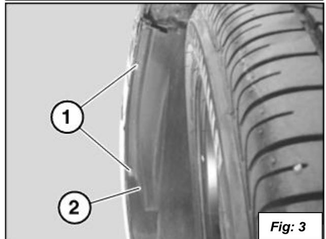
6. Pry the inner fender (1) out of the way and remove the two screws (2) holding the bumper to the fender. See figure 4.
