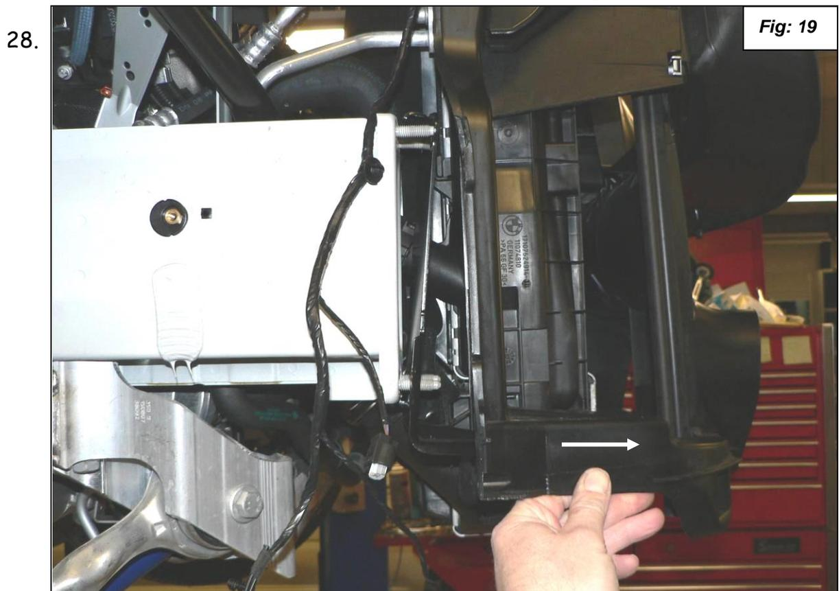
28. Slide the supplied new BMW part number 51 64 7 154 546 lower radiator support bracket with mount for oil cooler onto the studs where the other one without the mount for oil cooler was. See figure 20. Install nuts, bolts, screws and radiator mount in reverse order of removal. Torque bumper nuts to 22Nm (16 ft-lbs.). You do not need to replace rivets.
