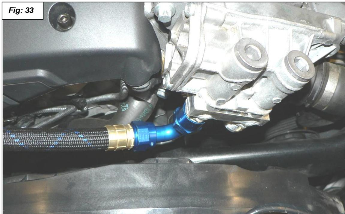
40. The straight end of the lower hose connects to the lower fitting of the oil cooler and the 45° fitting end connects to the adapter block onto the oil filter thermostat housing as shown in figure 34.
