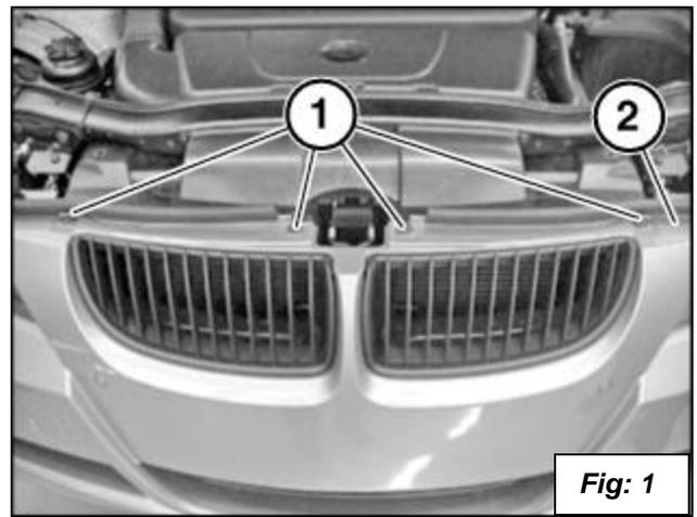
4. Remove the front inner fender on the right side by removing the screws at location (1) and (2). Unscrew the nut at location (3). Remove the Air Guide (4). Disconnect the connector from the tire pressure box. See figure 2.
