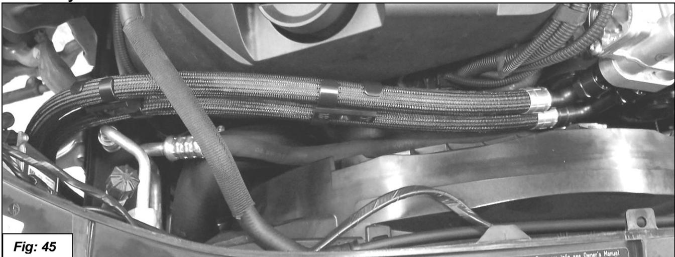
37. Install the 90°-swivel end of Upper Oil Line onto the adapter as shown below. Tighten the fittings in a position that the fittings and hose do not rub on anything that has a sharp edge. **Tighten fittings with 2 wrenches, one on hose fitting and the other on fitting attached to adapter block. Be sure to not loosen the adaptor fitting in this process!**
