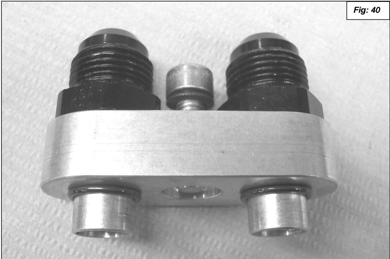
30. Install the oil line adapter block onto the oil filter thermostat housing. Make sure the O-Rings don't get pinched as you install the block. Torque the bolt to 20Nm (15ft-lbs.). See **figure 41**.
