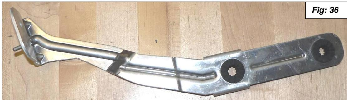
26. Install the top support bracket onto the new Dinan oil cooler mount with the supplied 6mm x 10mm bolts and large diameter flat washers. Install the rubber mounts and metal inserts, and attach lower mounting tab with the included hardware. Install the edge guards in the three places shown. See **figure 37**.
