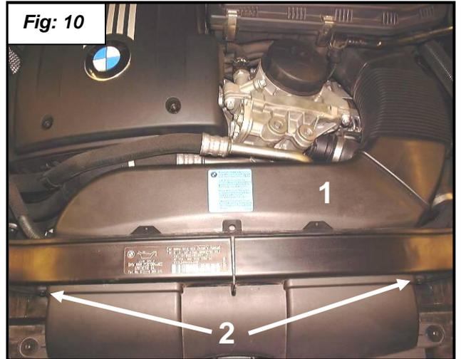
16. Remove the oil lines (1) from the oil filter control housing by removing the bolt marked with an arrow. Put rags under oil lines to catch oil (keep the oil off of the belts!). **See figure 11. Tip:** Use a flex head ratchet and you don't have to remove the fan cowl.
