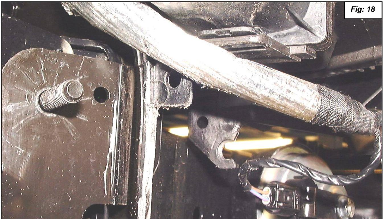
22. Remove the top support bracket from the stock oil cooler. The screws are tamper proof torx. If you do not have the correct tool to remove them, vise grip pliers will work in a pinch. **See figure 19.**
