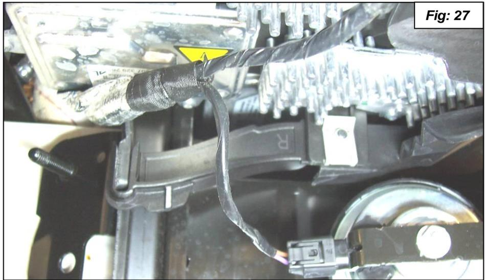
30. Install the Dinan headlight support bracket in place of the BMW bracket you removed in step 20. It fits between the headlight mount and the upper mount you did not cut off in step 20.
