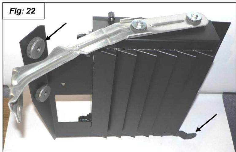
25. Replace the AC Line Support Bracket. To make room for the new Oil Cooler Hoses you will need to remove the stock plastic AC line support bracket from the front of engine. This bracket will be replaced by a new steel AC Line Support Bracket that relocates the AC line down and slightly forward. Pull the AC line out of the C-shaped tip of the stock support bkt. Remove bracket and save the single mounting bolt for the new support bracket. **See figure 23.**
