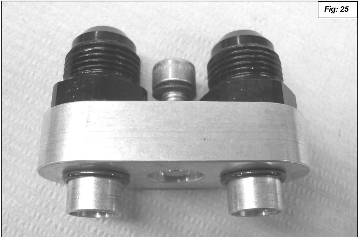
28. Install the oil line adapter block onto the oil filter thermostat housing. Make sure the O-Rings don't get pinched as you install the block. Torque the bolt to 20Nm (15ft-lbs.). See **figure 26**.
