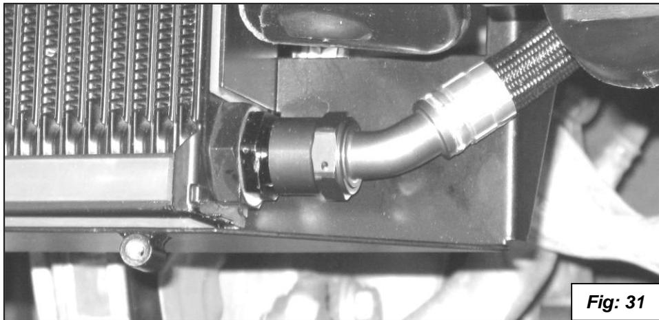
37. Tighten the upper fitting so the fitting is centered between the headlight and the cooler support bracket. It is best to use one wrench on the line fitting and one on the Oil Cooler hex to protect the Oil Cooler.
