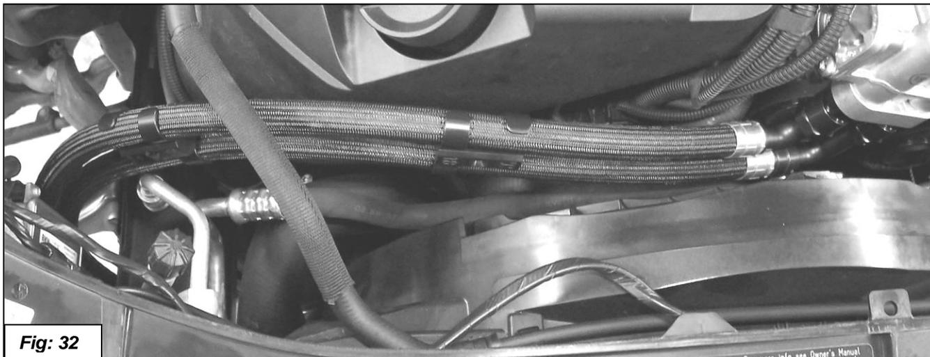
39. Install the 90°-swivel end of Upper Oil Line onto the adapter as shown below. Tighten the fittings in a position that the fittings and hose do not rub on anything that has a sharp edge. **Tighten fittings with 2 wrenches, one on hose fitting and the other on fitting attached to adaptor block. Be sure to not loosen the adaptor fitting in this process!**
