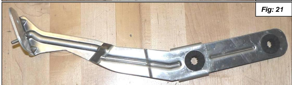
24. Install the top support bracket onto the new Dinan oil cooler mount with the supplied 6mm x 10mm bolts and washers. Install the rubber mounts, and attach lower mounting tab with the included hardware. **See figure 22.**
