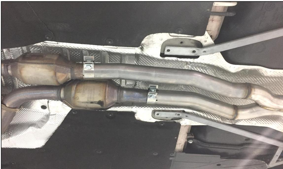
10. Slide the 2 muffler clamps forward onto the midpipe and reinstall the clamp hardware.
