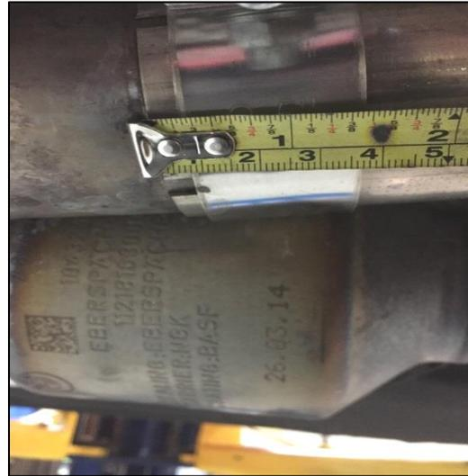
13. Rotate and position the muffler clamps as shown, and torque clamps to the specs below. Remove screw jack.:
