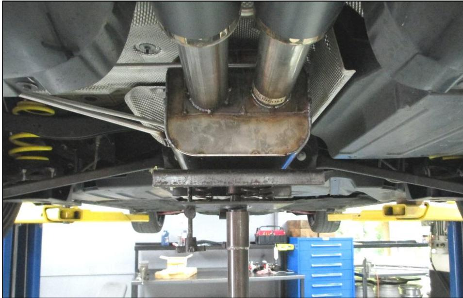
6. Insert the hanger rods on the DINAN muffler into the stock rubber hangers.
