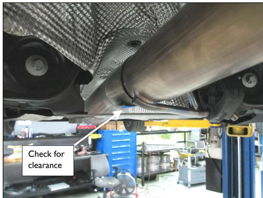
10. Be sure to check for proper clearance between the exhaust tips and bumper.
