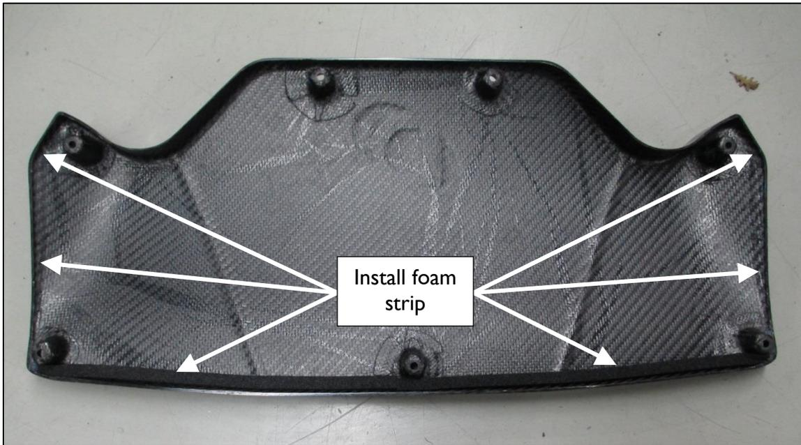
8. Place the Dinan lid onto the airbox. Be sure there is no foam strip visually exposed once the lid is installed, as shown in the next two figures.
