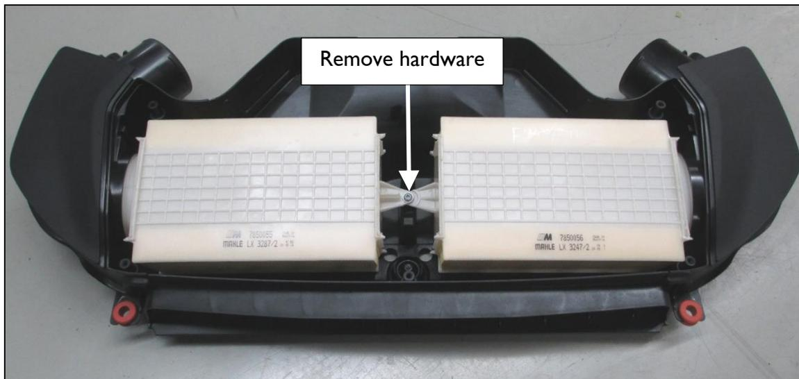
3. Remove the factory air filters.
