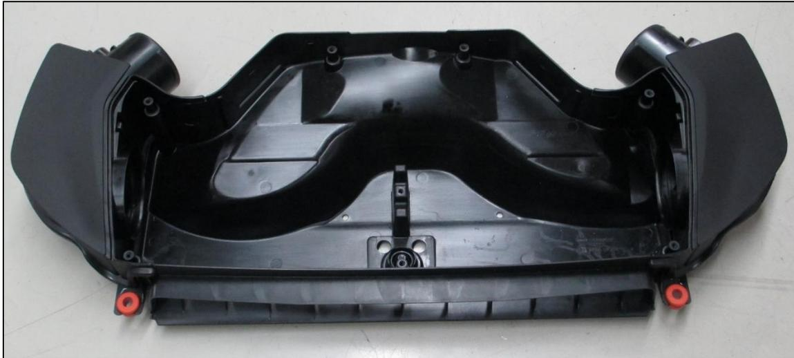
4. Install the Dinan air filters as shown. The open end of the Dinan air filters will slide inside the oval openings in the air box. The rubber "block" on the air filter cap points downward and helps hold the filters away from the air box bottom.
