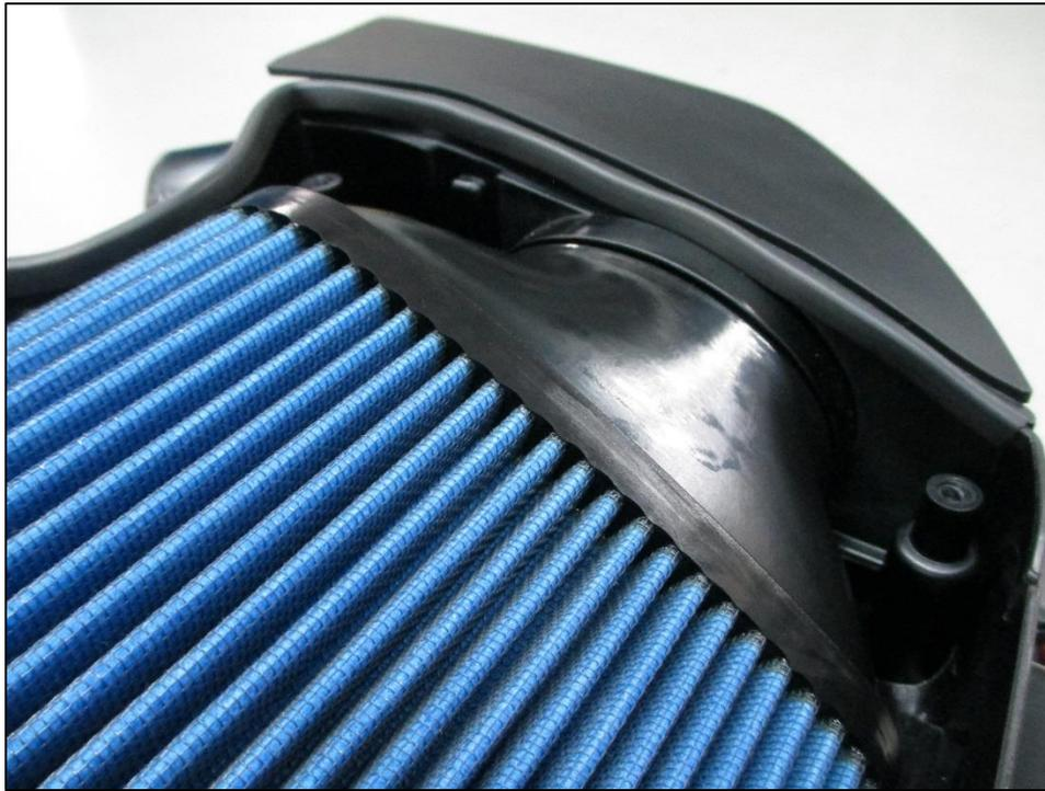
7. Install the supplied foam strip along the undersides of the front edge, and both sides, of the carbon fiber Dinan airbox lid as shown. Trim the length of the foam strip to fit as needed. Do not add foam to the rear edge.
