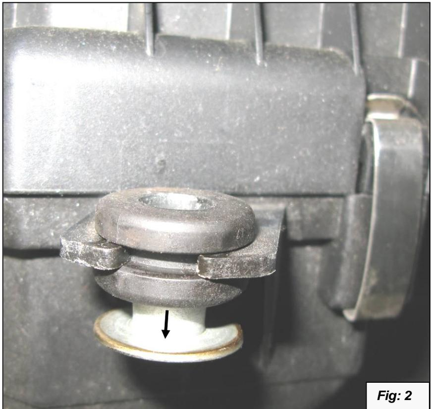
6. The passenger side front mount is different; the rubber mount there is attached to the car and is left on the car and mounted as stock.
