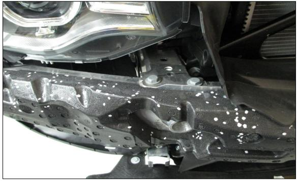
4. See photos below. Remove the lower air duct by unclipping the 6 tabs and 2 push pins.
