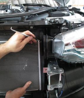
9. With the cooler removed, use a small grinder to remove the 2 tabs on the driver's side as shown.
