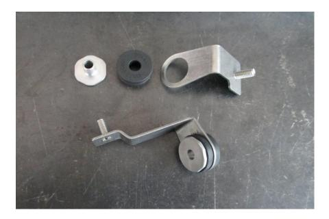
11. Using the included bolts and wave washers, install the brackets onto the Dinan cooler. Note that each bracket is unique, and must be positioned as shown.
