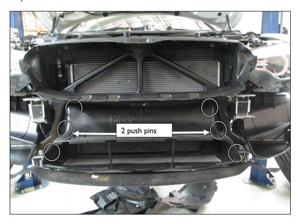
5. Remove the 6 bolts that secure the front brace (the top 2 bolts come in from the top of the car), and remove brace from vehicle. Take care to prevent damage to the fins on the after-cooler as you slide the brace past the upper air duct.
