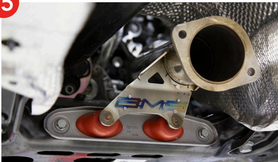
16. From the top of the car, align the factory V-band on the turbo outlet and loosely install the clamp. Make sure the downpipe can still move slightly and rotate.
