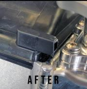
MUST BE TRIMMED FOR PROPER CLEARANCE OF THROTTLE BODY Y-PIPE FLANGE CONNECTION (APPROXIMATELY .5" / 12.5MM)
