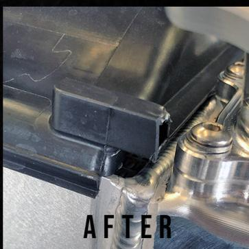
MUST BE TRIMMED FOR PROPER CLEARANCE OF THROTTLE BODY Y-PIPE FLANGE CONNECTION
