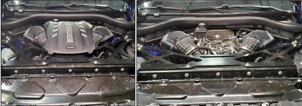
2. Remove all the push rivets and bolts holding the plastic cover, as shown. Repeat on other side as well. The sealing gasket shall be unclipped on both sides as shown below in order to properly raise the plastic cover. This operation will allow access to bolts needed in upcoming steps.
