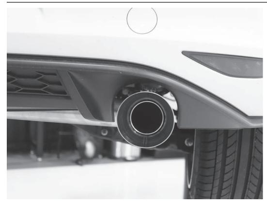
23) Adjust the exhaust tips to your desired position before tightening the pinch clamps to 55Nm (40 lb-ft). Verify tip is securly in place.
