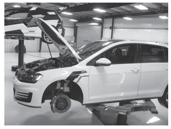
1) Securely lift vehicle. If a vehicle lift is not used, secure the vehicle with jack stands. It is not necessary to remove the wheels, but will make installation easier.
