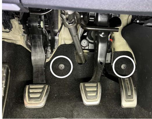
**STEP 6** - Locate the APP connector on the throttle pedal. Then, pull up on the red locking tab and squeeze/press it to disconnect the connector. Plug the PCU harness inline of the throttle pedal and throttle pedal harness.
