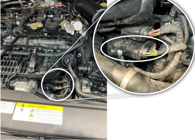
**STEP 11** - Using a pick tool, pull the red lock tab out and squeeze the release tab to disconnect the connector. Then plug the PCU harness inline of the engine harness.
