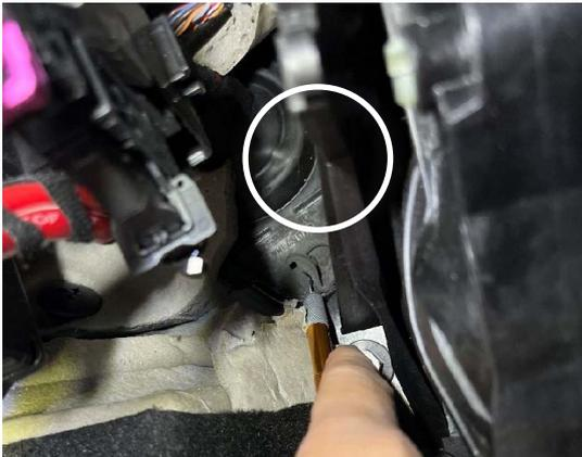
**⚠ CAUTION:** Please be careful when cutting an opening in the grommet, as the vehicle's electrical harnesses are only a few inches away from the grommet location.
