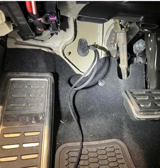
**⚠ CAUTION:** Please be careful when cutting an opening in the grommet, as the vehicle's electrical harnesses are only a few inches away from the grommet location.
