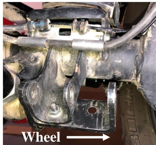
**Figure 13 – Passenger Side Offset Bracket**
