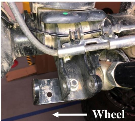
**Figure 12 – Driver Side Offset Bracket**
