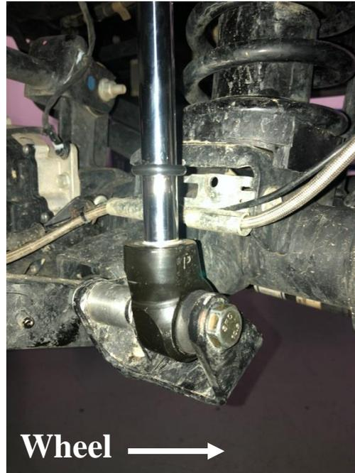
Figure 14 – Driver Side Bottom Mount    Figure 15 – Passenger Side Bottom Mount
