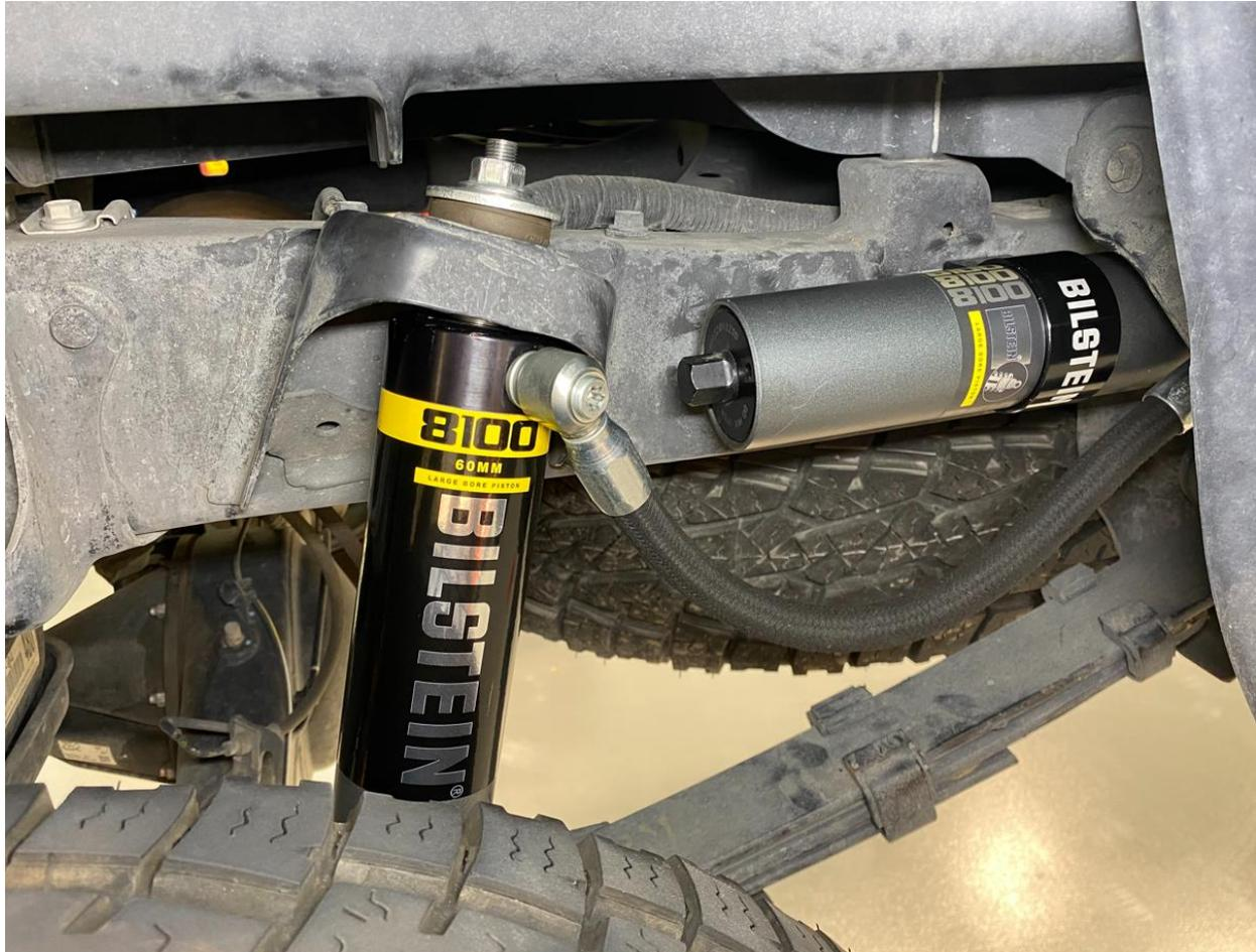
**Final right rear (passenger) B8 8100 shock installed on vehicle**
