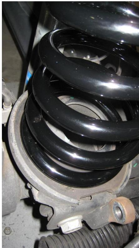
**Figure 5. Passenger side (pictured with Bilstein 5100 shocks)**
