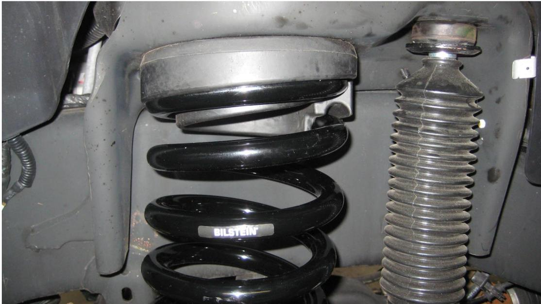
**Figure 6. Driver side (pictured with Bilstein 5100 shocks)**
