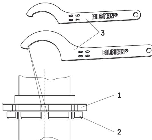
Fix the spring plate (1) and locknut (2) by using hook wrench (3) delivered by BILSTEIN.
