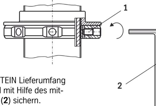
Fix the spring plate with the set screw (1) by using hex key (2) delivered by BILSTEIN.
