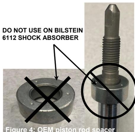
Figure 4: OEM piston rod spacer
