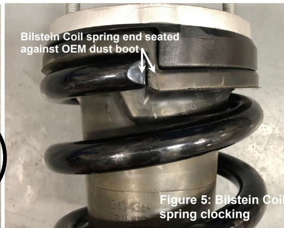
Figure 5: Bilstein Coil spring clocking
