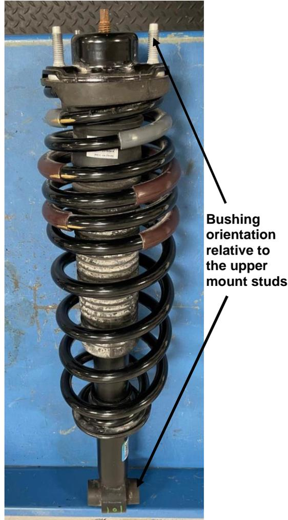
**Figure 1: OEM Bushing/spring**
