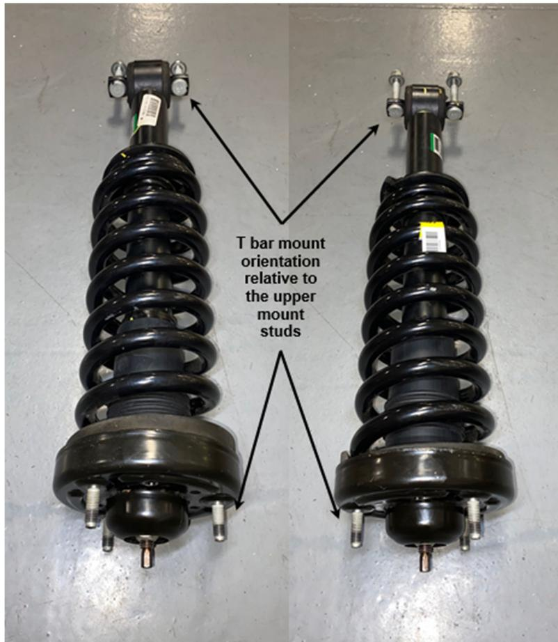
Figure 2: OEM T Bar Orientation
