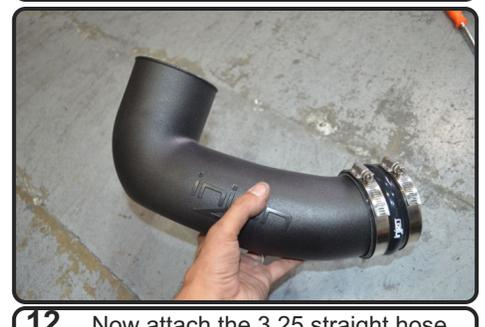
**12.** Now attach the 3.25 straight hose to the upper intake tube with clamps provided. Tighten the clamp on upper intake tube only.
