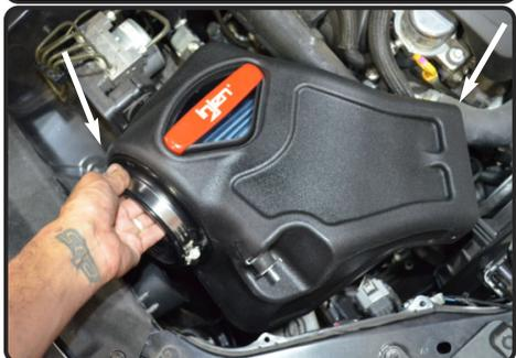
**21.** Install the air box into position. Attach the filter to the intake tube. Do not tighten.
