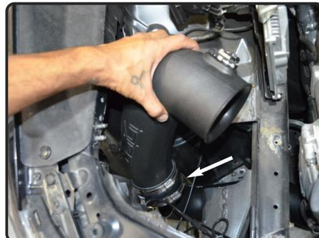
**14.** Install the upper intake tube to the lower intake tube and position.
