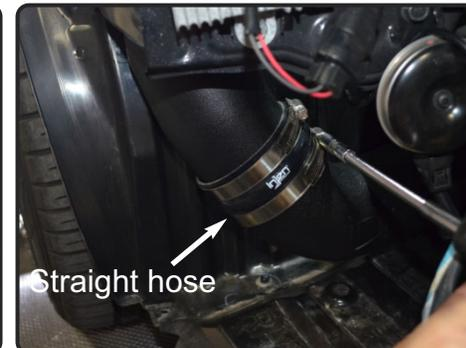
**15.** Position and snug fit the clamps both on turbo and straight hose. Do not tighten completely. Allow for adjustment if necessary.
