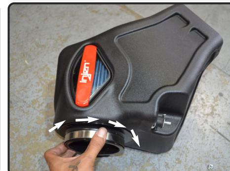
**19.** Once seated correctly, rotate filter in either direction a 1/4" turn till locks.
