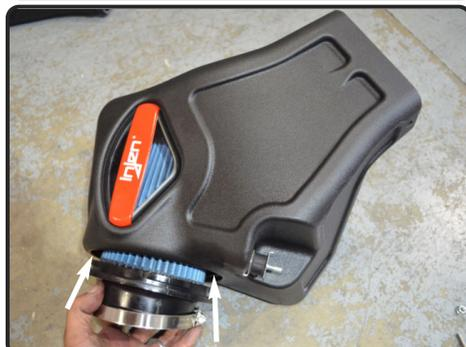
**18.** Install the twist lock filter into the airbox.
