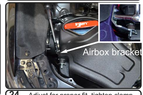
**24.** Adjust for proper fit, tighten clamp using 8mm nut driver. Secure the box using the OEM bracket and hardware from step 3. Secure and tighten.
