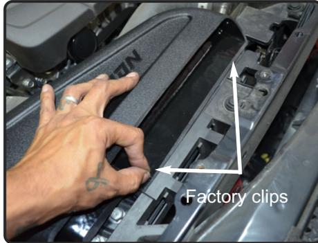
**28.** Re-install the factory retaining rivets from step 2. to the injen scoop and secure. Re-install bumper cover and Re-connect Battery.
