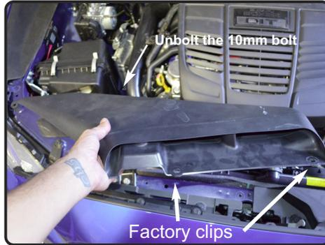
**2.** Remove the two plastic retaining rivets from the air scoop and remove scoop from engine bay. Save for later install. Loosen the 10mm bolt holding in the lower part of the air box to the vehicle frame.
