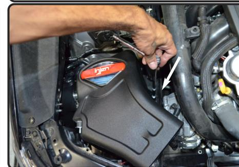
**23.** Once intake system is in position from step 20, tighten and secure the box to the vehicle frame using 10mm socket or wrench.
