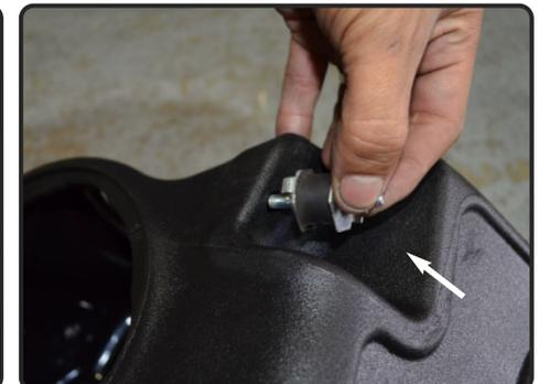
**16.** Install the OEM isolation mount from step 3.
