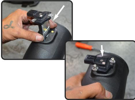
**13.** Install the MAF sensor into the new injen intake tube, secure and tighten using provided M4 button head screws.
