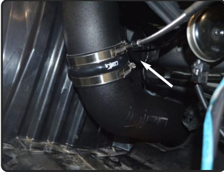
**25.** Now secure and tighten all clamps on the intake system using 8mm nut driver.
