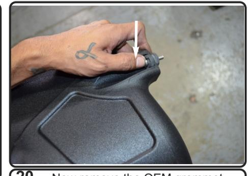
**20.** Now remove the OEM grommet and crash washer screw out of the OEM air box. Install to the bottom of the air box. Secure to the airbox.
