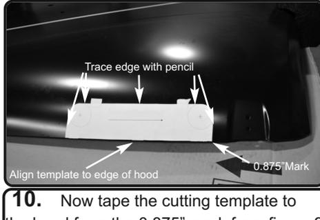
10. Now tape the cutting template to the hood from the 0.875" mark from figure 9 and make sure you line up the bottom of the cutting template to the edge of the hood. Use a pencil and trace the edge of the template for a cutting guide for the next step.
