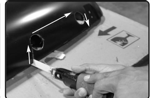
12. The line drawn from the template in figure 10 will be a guide to cut using an air saw to cut a straight line. **Please use caution and cut slow!!!**
