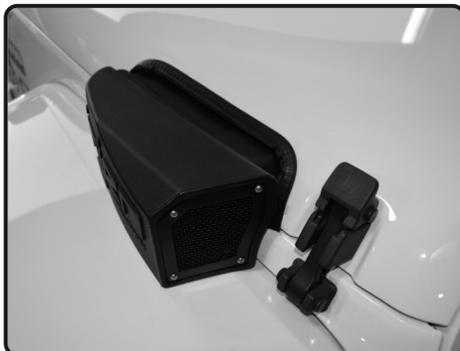
**17.** Close the hood and make sure the cut out clears the scoop, grind back some more if more clearance is desired.
