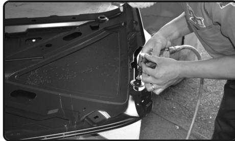
**14.** Use a flat grinder to straighten the edges and clean up all the metal burrs. Slowly grind back on the open. Only grind what you need for additional clearance. ***Please use caution and have proper safety equipment like goggles and air respirator!!!***
