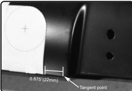
9. Locate the hood latch indentation and make sure you line up the bottom of the cutting template to the edge of the hood. Use a pencil and trace the edge of the template for a cutting guide for the next step.
