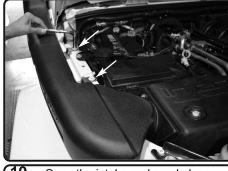
**19.** Once the intake and snorkel are re-installed, re-use the two factory 10mm bolts removed from figure 16 and secure the bracket on the snorkel to the fender.
