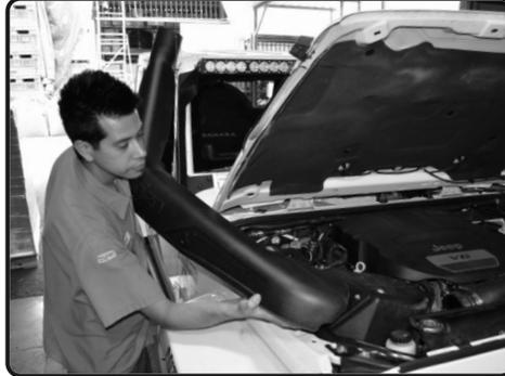
**18.** Re-install the Injen air box with the Injen snorkel attached to it.
