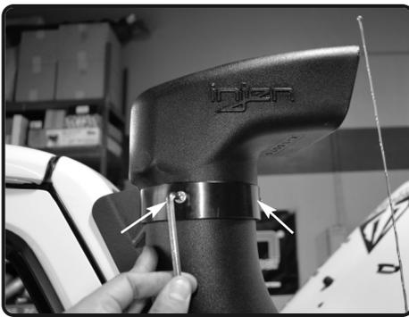
**21.** Install 3- M6 allen bolts and washers to secure the snorkel scoop to the snorkel.
