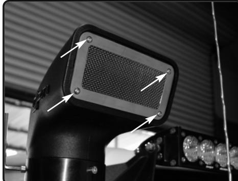
**22.** Use 4-M4 bolts to secure the mesh screen to the snorkel scoop
