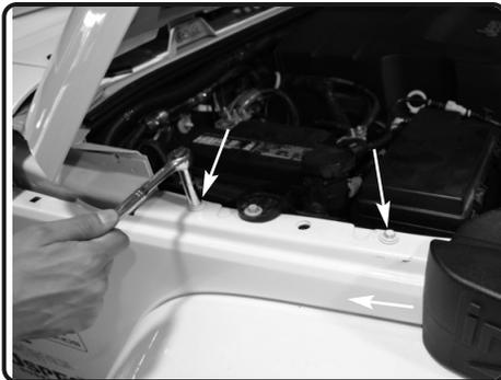
**17.** Remove the 2-10mm bolts on the fender.
