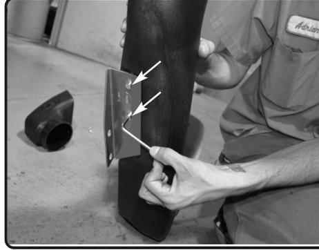
**15.** Install the A-bracket onto the side of the snorkel and secure it with 2-M6 allen bolts
