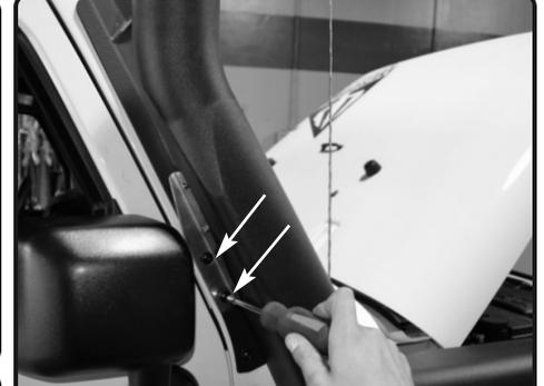
**20.** Re-use the 2 factory torx bolts and secure the A-bracket to the window pillar
