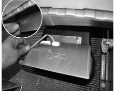
Install the rain guard. Secure using provided M6 socket cap screws and tighten. Once secure, cover the socket cap screw using provided vinyl cap. This will prevent any contact with screws and front bumper support. Failure to do so will result in vibration noise.
