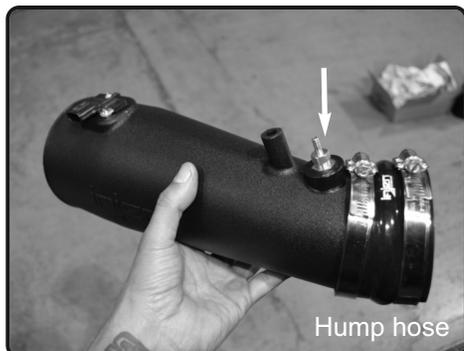
**13.** Install the 1/8" NPT fitting, to the insert on intake tube and secure. Install the 3-1/2" hump hose with clamps provided to the intake tube.
