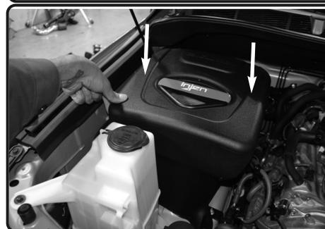
11. Place the Injen air box assembly into the engine bay and line up the pegs below the Injen air box to the vibramounts.
