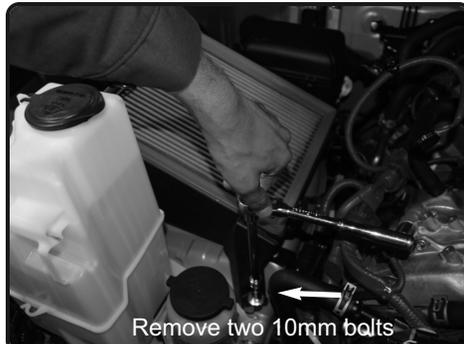
6. Locate the 2 bolts holding in the bottom half of the air box, loosen and remove.
