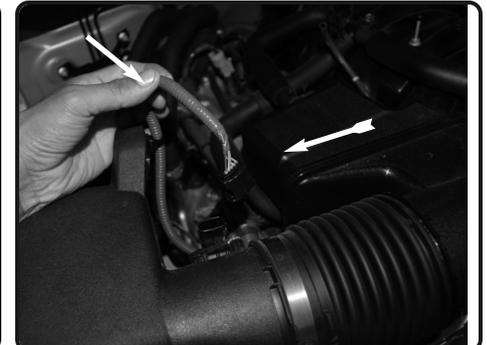
4. Disconnect the MAF sensor harness. Pull harness from the air box.
