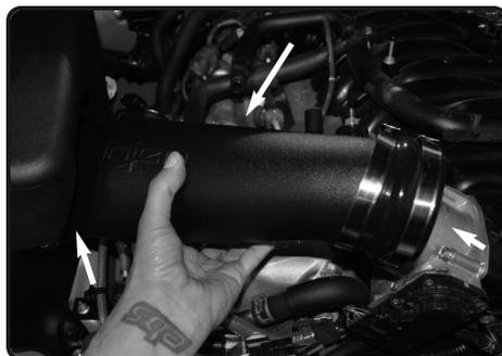
**14.** Insert the Injen intake tube assembly to the vehicle.
