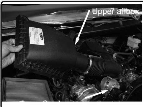
5. Unclip the upper half of the air box assembly and remove from the vehicle.
