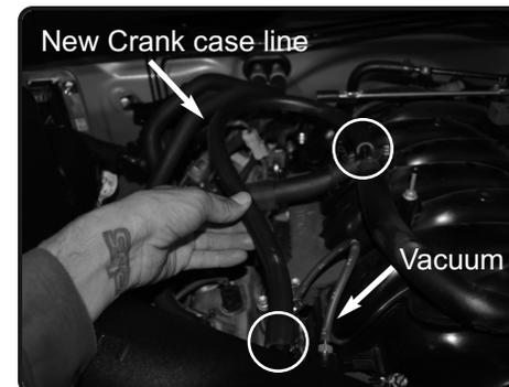
**16.** Reconnect the vacuum line to the fitting on intake tube. Install provided 12mm crankcase hose and secure to the intake tube and engine.
