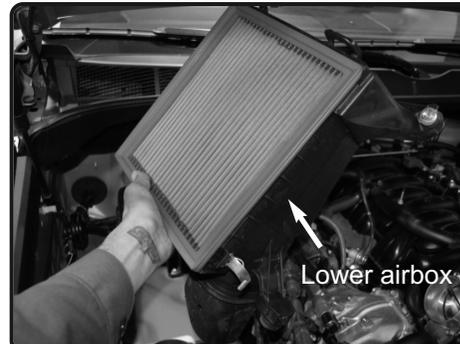
7. Remove the bottom half of the air box out of the vehicle.
