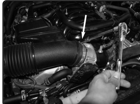
2. Lift up firmly to remove the engine cover. Loosen the clamp on throttle body using 10mm socket and ratchet.
