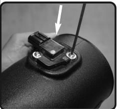
12. Remove the MAF sensor from stock intake tube. Install into the new injen tube using provided M4 button head screws.
