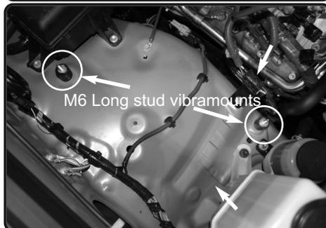
10. Using the OEM mounting locations, install provided long stud vibramounts to the threaded inserts. **Make sure the long stud is facing up. short side is secured.**
