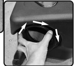
8. 1) Insert twist lock filter to the air box. 2) Once seated, rotate in either direction 1/4 turn till filter locks.
