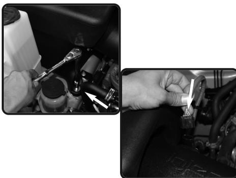
**17.** Secure the box and tighten using 10mm socket and wrench. Re-connect MAF sensor harness.
