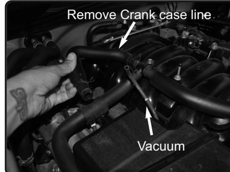
3. Disconnect the small vacuum line and remove the crank case line from the air box and engine.
