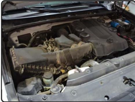
**1.** Stock intake system shown. Lift up engine cover and remove.
