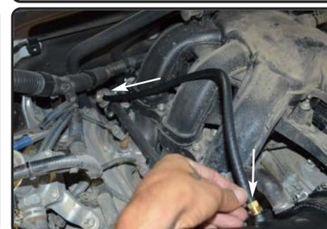
**23.** Remove the smaller vacuum line, install the provided 4mm vacuum line and secure to engine and fitting on intake tube. Re-install the engine cover.
