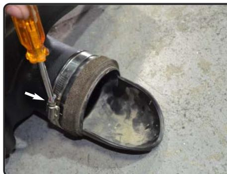
**14.** Secure using provided #56 band clamp.
