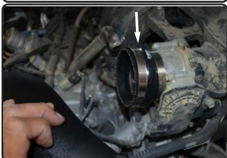
**20.** Install step hump hose to the throttle body. Install the intake tube to the vehicle and position.
