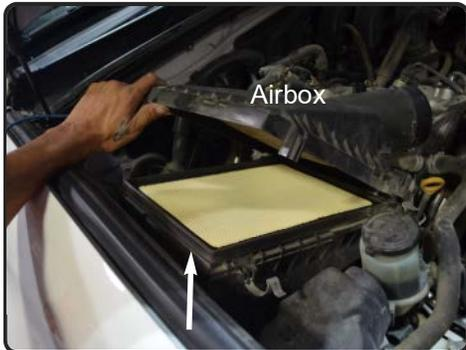
**4.** Unclip upper half of airbox and remove from vehicle.
