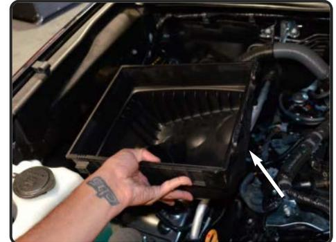
**7.** Now lift up and remove the lower part of the airbox out of vehicle.
