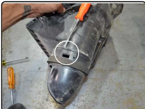
**12.** Carefully remove the OEM Air box scoop using flathead screwdriver.
