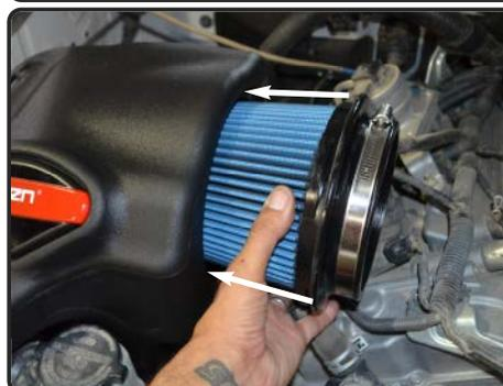
**18.** Insert twist lock filter to the air box.
