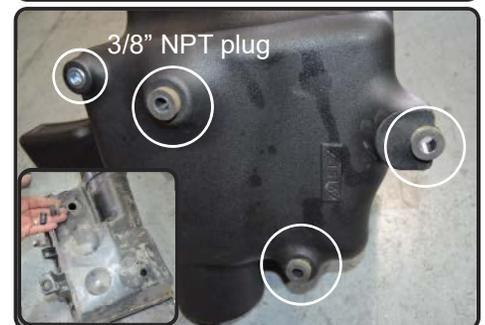
**11.** Remove the 3 grommet with crush-washer and install into the new air box. Install the provided 3/8" NPT plug to the threaded hole on the air box.
