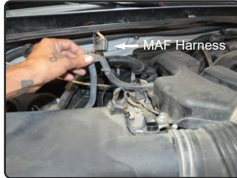
**2.** Disconnect the MAF sensor harness and pull line away harness from the airbox.
