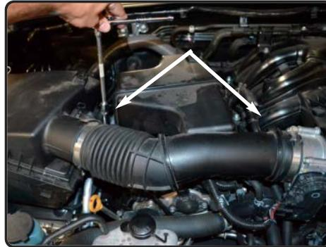
**7.** With 10mm nut driver or socket with ratchet, loosen the clamps on throttle body and airbox.
