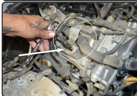
**10.** Loosen and remove the harness bracket from the engine using 10mm socket or wrench.
