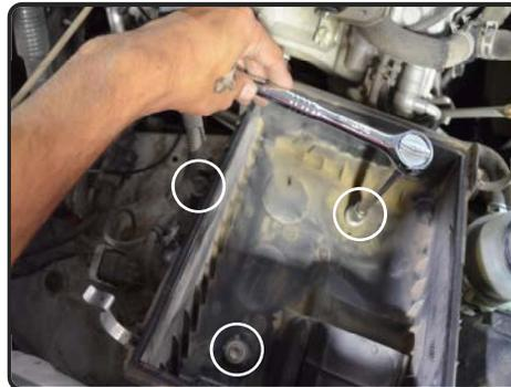
**6.** Loosen the 3 bolts holding in the lower part of the airbox.
