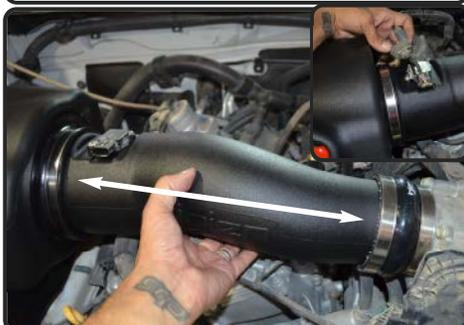
**21.** Once adjusted and positioned properly, tighten all clamps using 8mm nut driver. Connect the MAF sensor harness.
