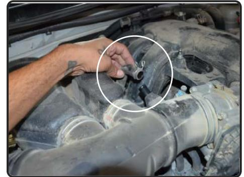
**3.** Now disconnect the Crank case fitting from the intake tube and pull back from tube.
