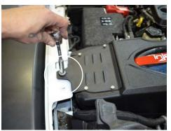
20. Tighten the bracket using the oem bolt 21. Secure and tighten all the clamps on from step 4.
