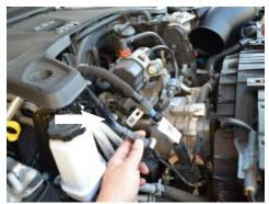
9. eTORQUE MODELS ONLY: Reroute the crank case line under the generator
