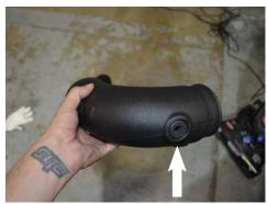
16. Install the provided rubber grommmet 17. Insert the Injen intake tube into the to the intake tube
