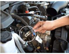
8. eTORQUE MODELS ONLY: Remove the nut holding down the generator harness and remove the harness from the bracket. harness.
