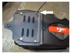
13. Secure the bracket to the air box using M6 socket cap screws.
