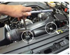
3. Remove the 2 bolts holding in the intake tube.
