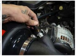
18. Connect the crank case vent tube vehicle. Position tube to the filter and step to the machined fitting on the intake tube.
