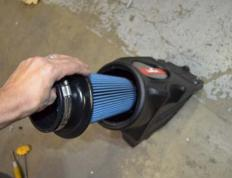
14. Install the twist lock filter on to the Injen air 15. Line up the airbox to the facotry box. Once seated, rotate the filter a 1/4 turn in either direction so the filter can lock into place. airbox using the OEM screw from step 4.
