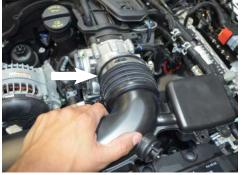
5. Loosen the clamp on the throttle body and pull back the intake tube from the throttle body.
