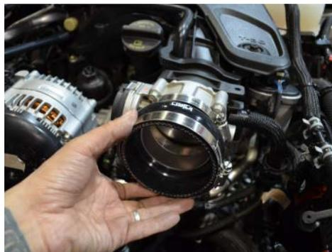
11. Install the provided step hump hose to the throttle body. Secure using provided clamps.
