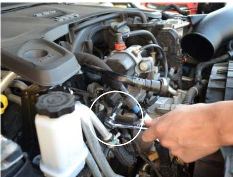
10. eTORQUE MODELS ONLY: Reattach the generator harness to the bracket then bolt down the generator harness.
