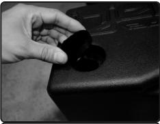
**7.** Place the filter minder plug into the filter minder hole on the air box assembly
