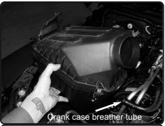
**5.** Disconnect the crank case breather tube. Then firmly lift up and pull the factory air box assembly out of the engine bay.
