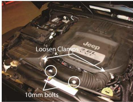
2. Remove the engine cover. Next loosen the two clamps from the intake tube. Finally, remove the two 10mm bolts.
