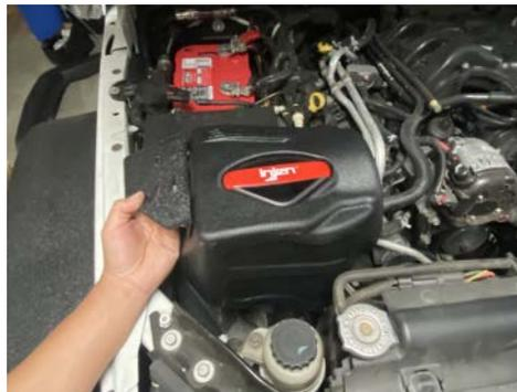
8. Install the Injen air box into the engine bay. Line up to the stock grommets and push down on the air box to secure.
