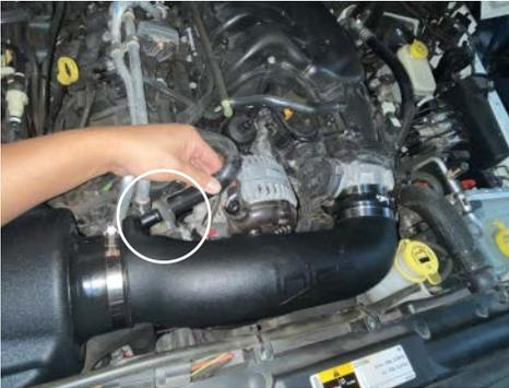
16. Reconnect the crank case breather hose to the injen tube.
