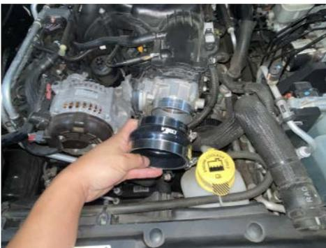
10. Place the hump hose onto the throttle body and secure using the provided clamps.
