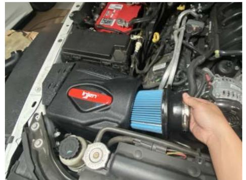
9. Install the twist lock filter on to the Injen air box. Once seated, rotate the filter a 1/4 turn in either direction so the filter can lock into place.
