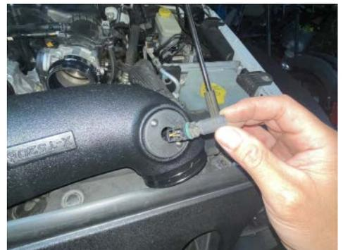
12. Install the IAT sensor to the adapter. Once fully seated, rotate the sensor to secure in place.
