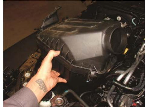
6. Remove the stock air box by firmly lifting it out of the engine bay.
