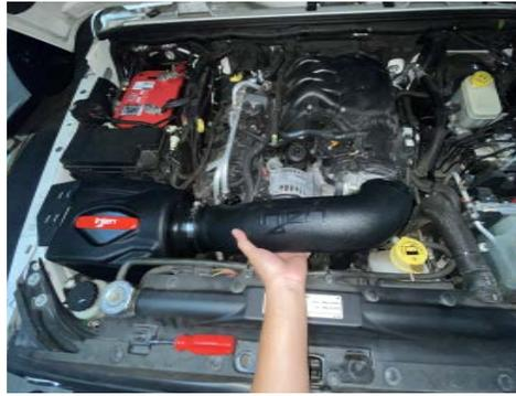
14. Insert the Injen intake tube into the vehicle. Position tube to the filter and hump hose.
