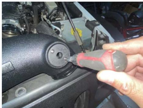
11. Place the temp sensor adapter onto the tube and secure using the provided M4 bolts.
