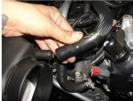
5. Disconnect the crank case breather tube from the stock air box.
