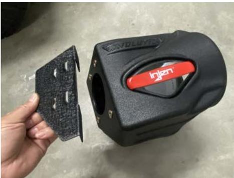
7. Bolt down the heatshield to the air box using the provided M6 bolts.
