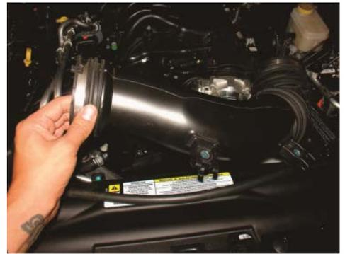
3. Disconnect the IAT harness and remove the intake tube from the throttle body and air box.
