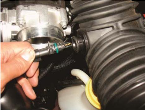
4. Twist the IAT sensor to remove the sensor from the intake tube.
