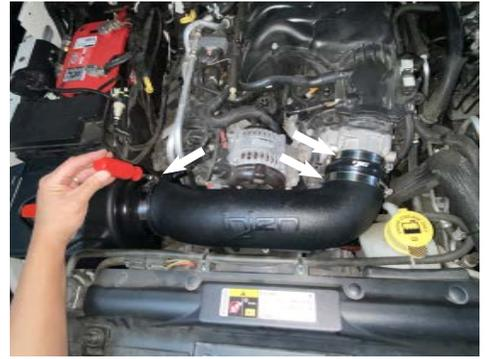
15. Secure the clamps on the filter and the hump hose.
