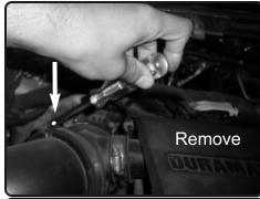
**3.** Loosen clamp on intake tube. Loosen the nut holding in the Duramax resonator box and remove. Lift up and remove the OEM air box out of vehicle.
