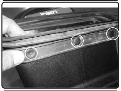
7. With original push clips, install and secure the front.
