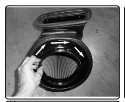
**12.** Once seated, rotate in either direction 1/4 turn till filter locks and is secured.
