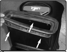
**6.** Place the seal on top and line up holes.
