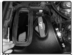
**14.** Make sure the injen air box is seated and secured properly into the OEM bracket. Make sure grommet from step 9 is locked in and seated in bracket.
