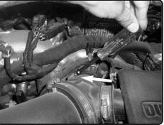
**2.** Loosen the clamp on turbo suing 8mm nut driver.
