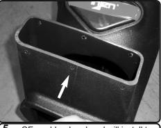
**5.** OEm rubber hood seal will install to the new injen air box.
