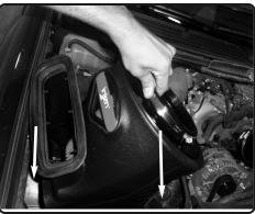
**13.** Install the injen airbox into the vehicle and position to the OEM air box location and secure.
