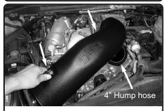
**16.** Install the provided 4" hump hose with clamps. Install the intake tube. (coolant line is optional to run on top or below intake tube) Positon intake tube.
