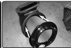
11. Insert twist lock filter to the air box
