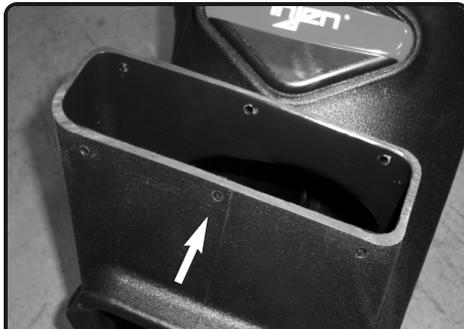
5. OEM rubber hood seal will install to the new Injen air box.
