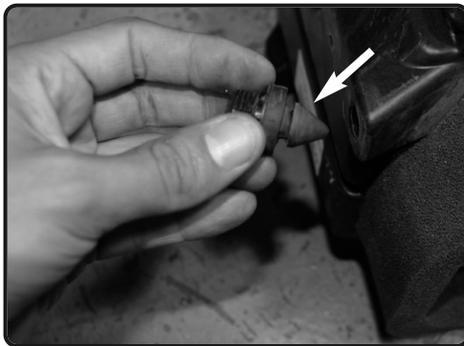
9. Remove the grommet lock spacer from the factory air box.
