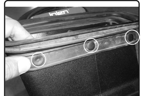
7. With original push clips, install and secure the front.
