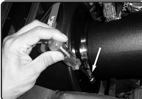
**16.** Adjust the tube for correct fit. Make sure the tube is bottom-out on filter. this will allow for the Rubber hood seal to seat properly. Secure and tighten using 8mm nut driver.
