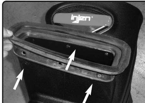
6. Place the seal on top and line up holes.
