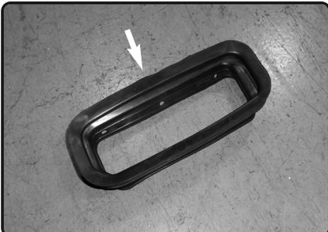
4. With pliers, loosen and carefully pull back push clips and remove the OEM rubber hood seal. Save clips and seal for later install
