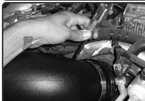
**18.** Secure and tighten the clamps on turbo using 8mm nut driver.
