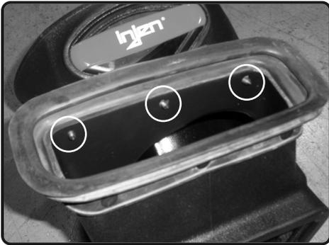
8. Install and secure the back side.
