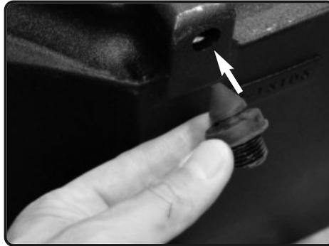
10. Now install the grommet lock spacer into the new Injen air box and secure.
