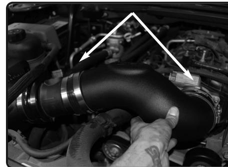
**23.** Install the intake tube. Position for best fit, secure and tighten all clamps using 8mm nut driver.
