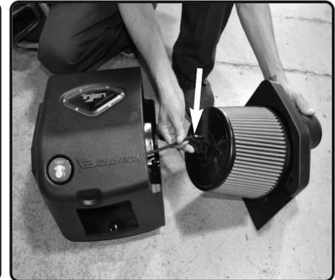
**3.** Connect the 3 mm Vacuum line to the 5/32" fitting on the top of the filter.
