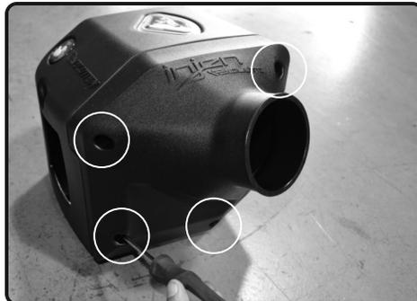
**17.** Now secure the plenum using provided 4 M6 screws and rubberized washers. Secure and tighten.
