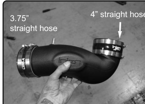
**18.** Install the the 4" and 3.75" straight hoses to the tube with clamps provided.
