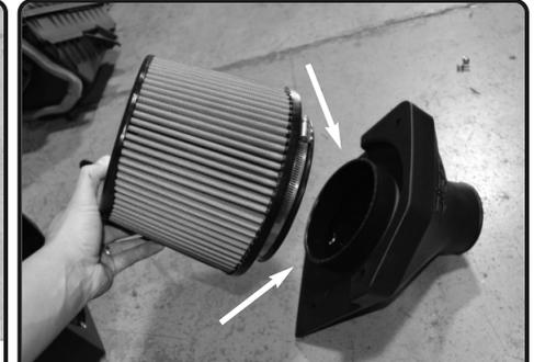
**16.** Install the filter to the plenum, secure and tighten using 8mm nut driver.
