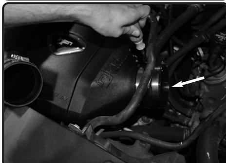
**21.** Install the 4" hump hose to the plenum. Tighten clamp on plenum only.
