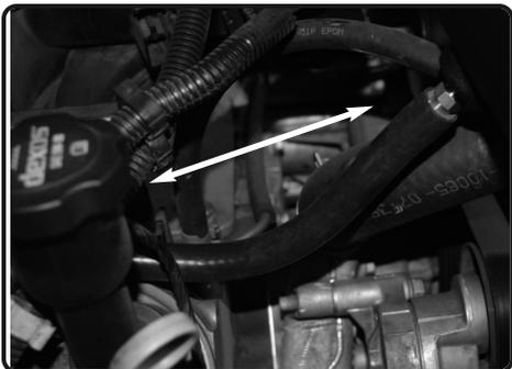
**25.** Install the provided 8mm hose to the crank case vent tube on engine, and connect the other end to the fitting on the intake tube.
