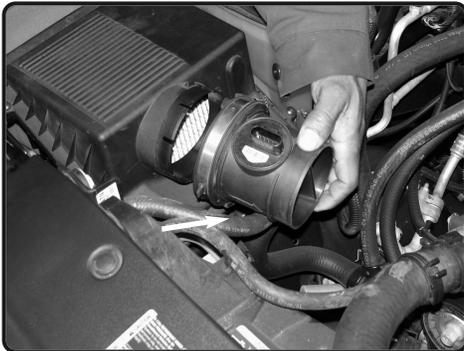
**5.** Loosen the clamp using 8mm nut driver. Remove the MAF sensor from air box. Remove the factory coupler from MAF sensor.
