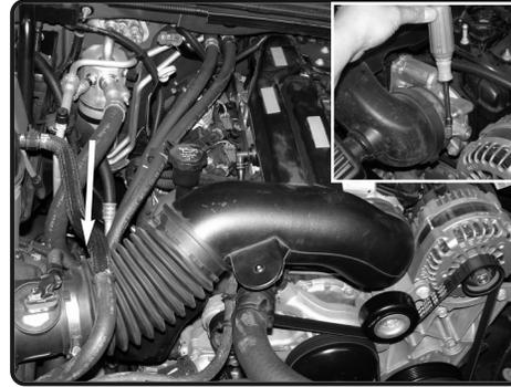
**3.** Use a 8mm nut driver and loosen the clamp on the intake air duct from the air box assembly and clamp on throttle body.
