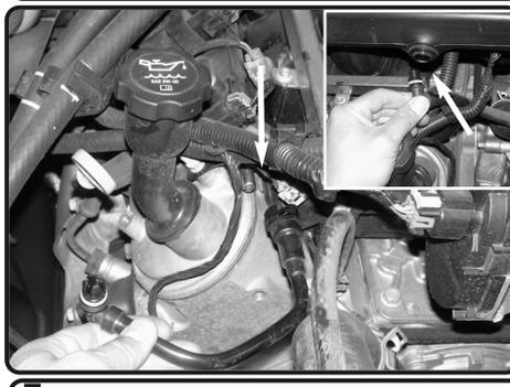
**7.** Disconnect the crank case ventilation line from the air duct resonator section located on top of the intake manifold. You will need to unclip a plastic lock in order for you to remove this line from the valve cover.
