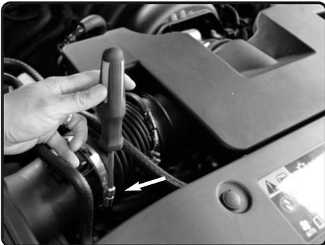
5. Loosen the clamp on the air box using 8mm nut driver.
