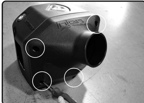
**18.** Now secure the plenum using provided 4 M6 screws and rubberized washers. Secure and tighten.
