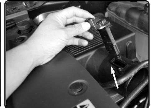
4. Pull the MAF sensor out of the factory air box assembly
