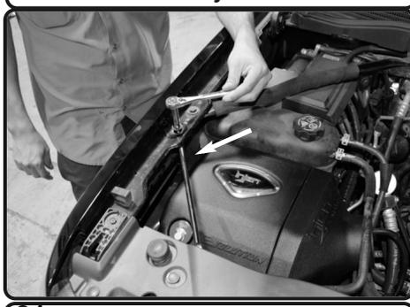
**21.** Secure the air box, re-secure the support bar.
