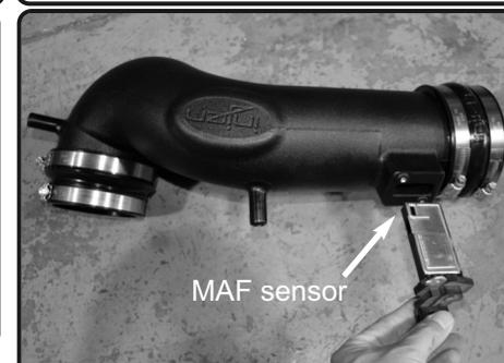
**18.** Install the MAF sensor into the intake tube and secure using provided M4 button head screws.
