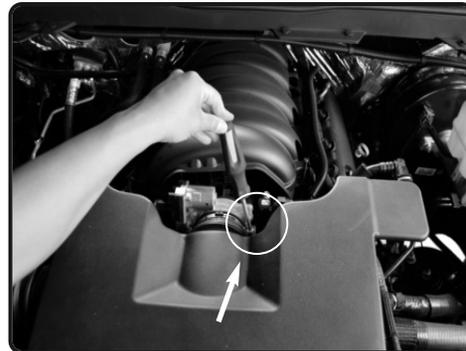
6. Loosen the clamp on the throttle body.
