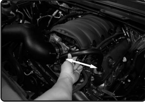
**24.** Install the provided 14.5" 15mm hose to the fitting on engine and intake tube on driver side.
