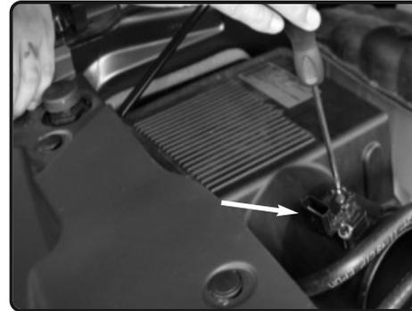
3. Use a T15 Torx bit and remove the two screws on the MAF sensor.
