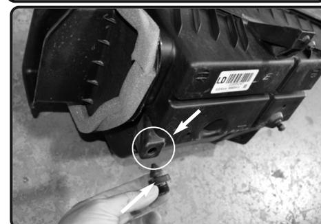
10. Remove the grommet spacer from the factory air box.
