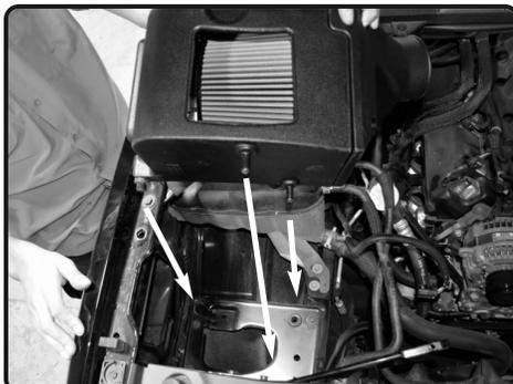
**20.** Now install the air box assembly into the vehicle. Position the tabs to seat like OEM box.
