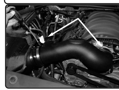
**22.** Install the intake tube. Secure the tube to airbox and throttle body. Position for best fit and tighten clamps. Re-connect the MAF sensor Harness.
