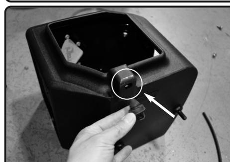
11. Now install the grommet spacer into the new injen air box and secure.
